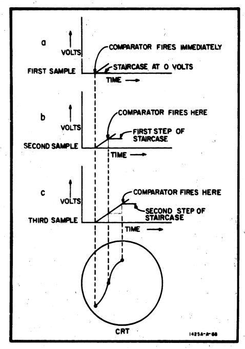
Figure 4-1. Comparator Operation
