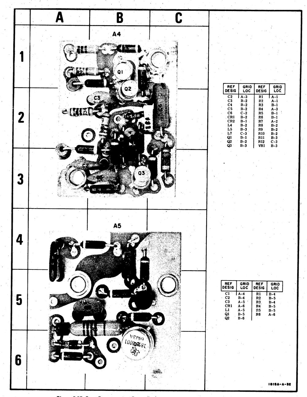
Figure 8-35. Step Generator and Power Source Assemblies A4 and A5 Parts Locations
