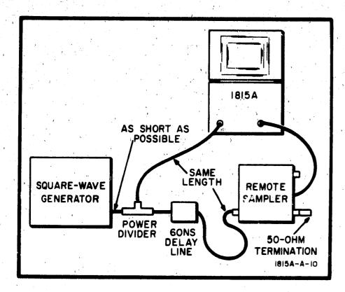
Figure 5-19. Minimum Delay Test Setup
