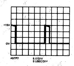
FIGURE 8-25. STAIRCASE AND BLANKING MEASUREMENTS
