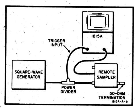
Figure 5-5. CW Triggering Test Setup
