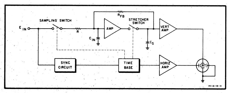
Figure 4-4. Complete Sampling System
