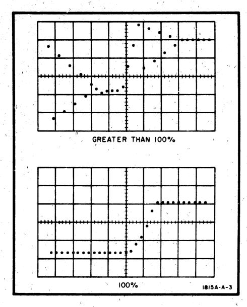
Figure 5-11. Sampling Efficiency Displays
