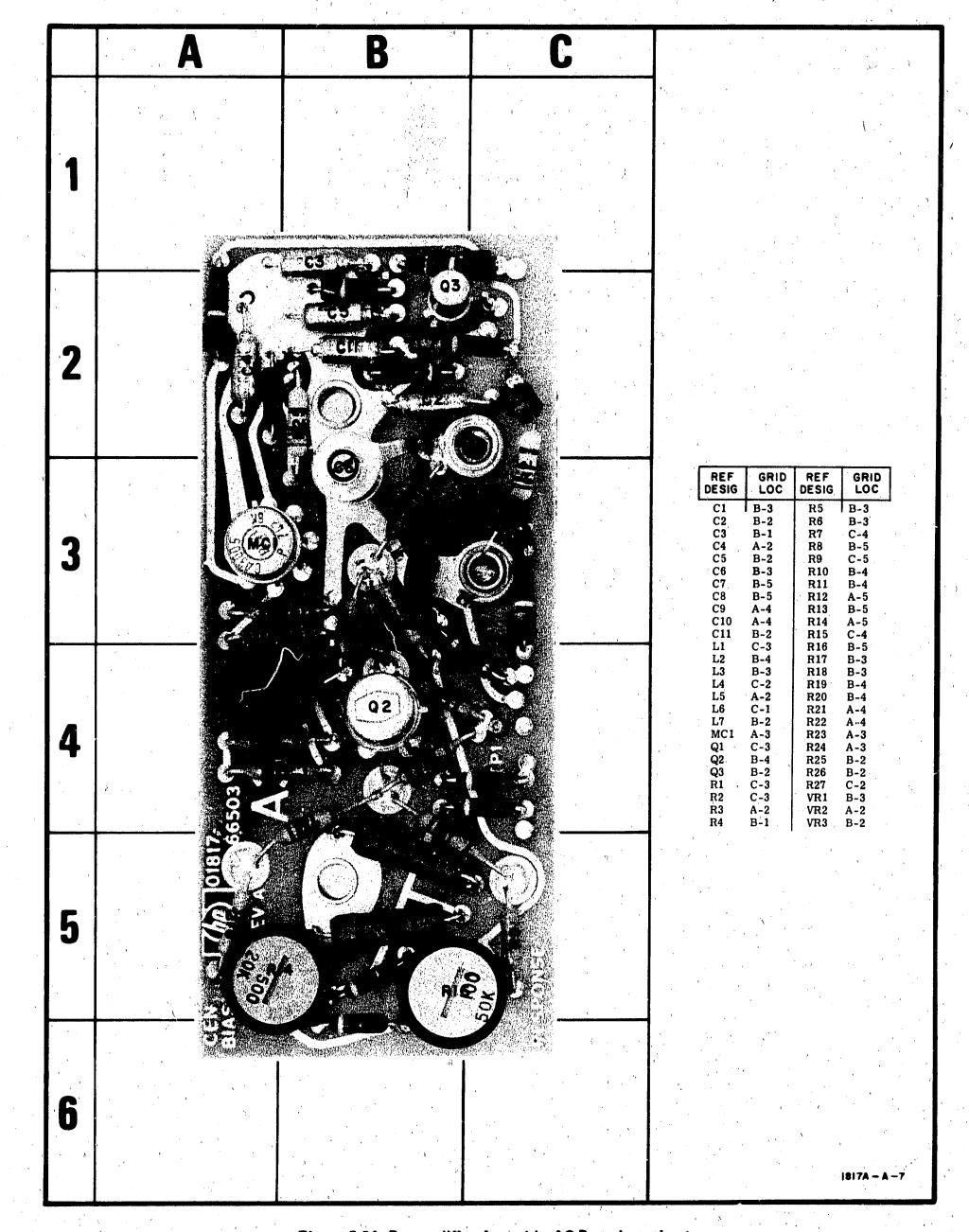
Figure 8-31. Preamplifier Assembly A3 Parts Locations
