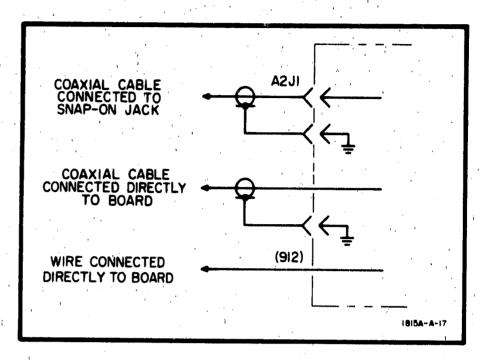
Figure 8-1. Circuit Board Connections
