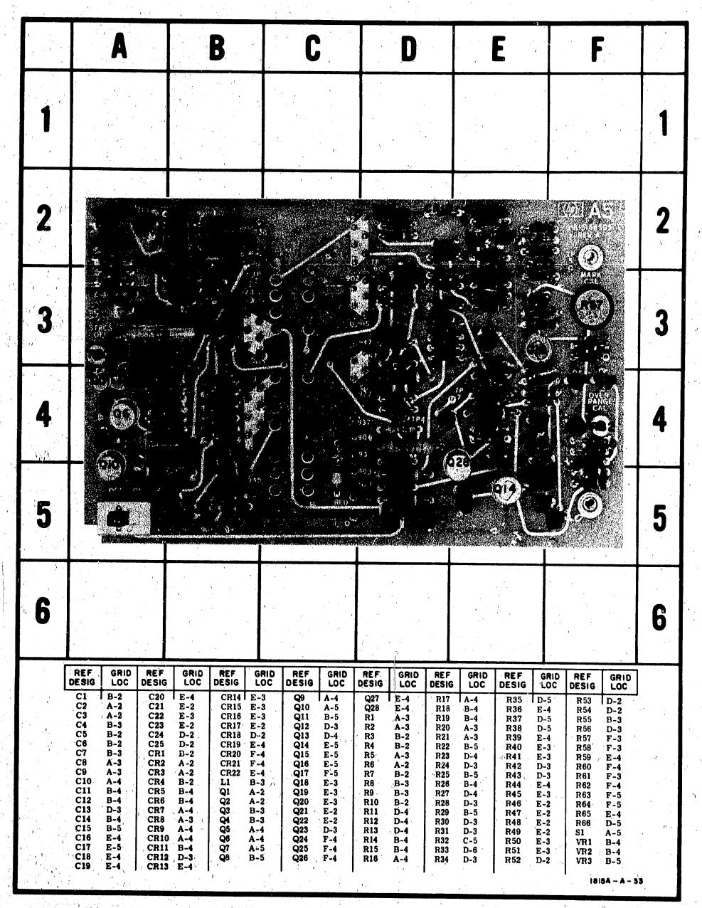
Figure 8-24. Staircase and Marker Dot Assembly A5 Parts Locations
