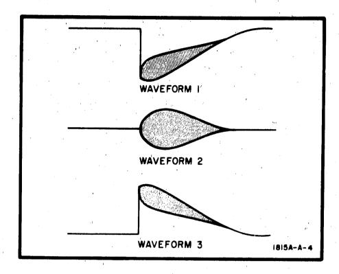
Figure 8-3. Diode Check Waveforms
