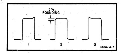
Figure 5-12. Low-frequency Distortion Waveforms
