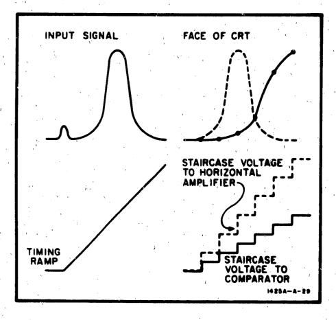
Figure 4-7. Staircase Attenuation
