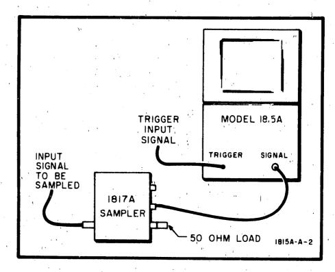
Figure 3-3. Sampling Operation Setup
