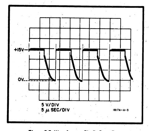
Figure 8-5. Waveform at Pin B, Step Reset
