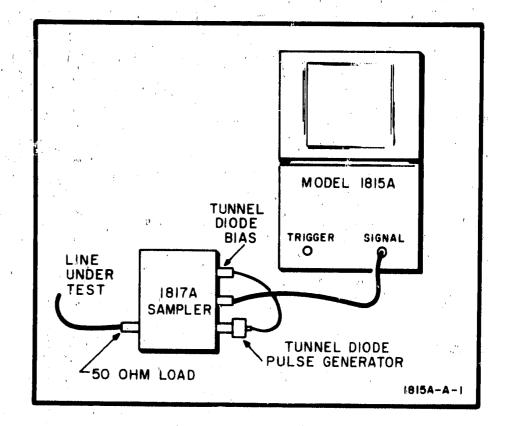
Figure 3-2. TDR Operation Setup
