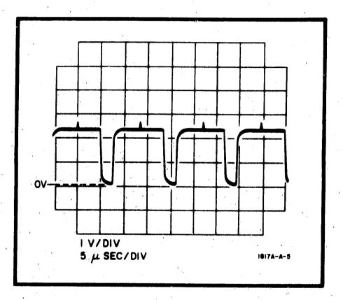
Figure 8-6. Model 1817A Output Waveform
