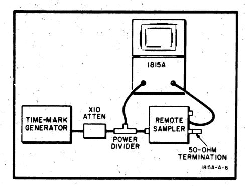
Figure 5-16. TIME/DIV Test Setup
