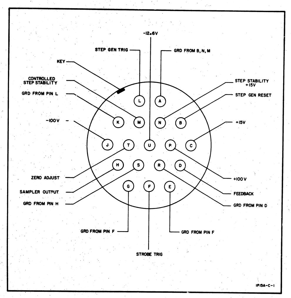
Figure 8-34. Sampler Cable Schematic
