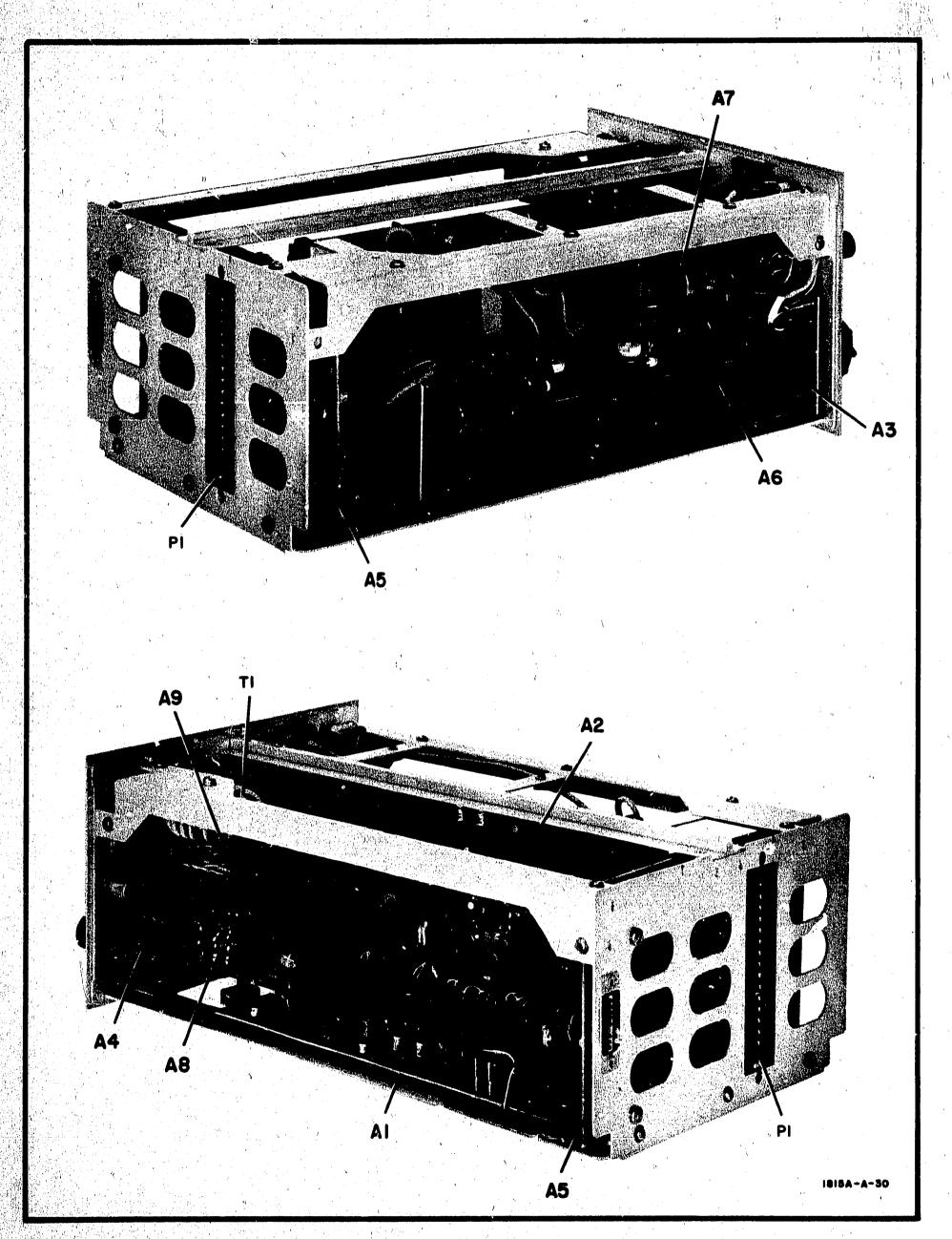
Figure 8-9, Model 1815A or B Assembly Locations
