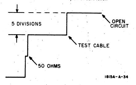
Figure 3-4. Vertical Axis Calibration
