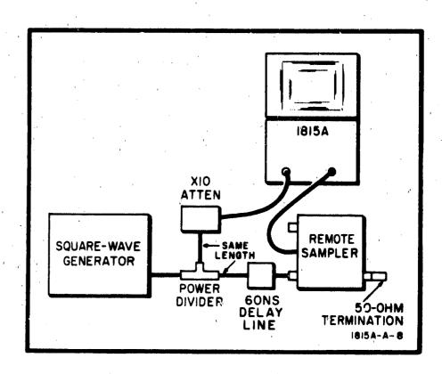
Figure 5-4. Pulse Triggering Test Setup
