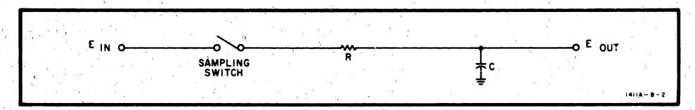
Figure 4-2. Basic Sampling Circuit
