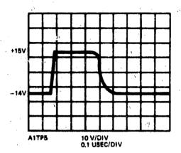
FIGURE 8-11, STRETCHER, VERTICAL AMPLIFIER MEASUREMENTS
