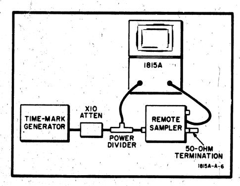
Figure 5-2. TIME/DIV Test Setup
