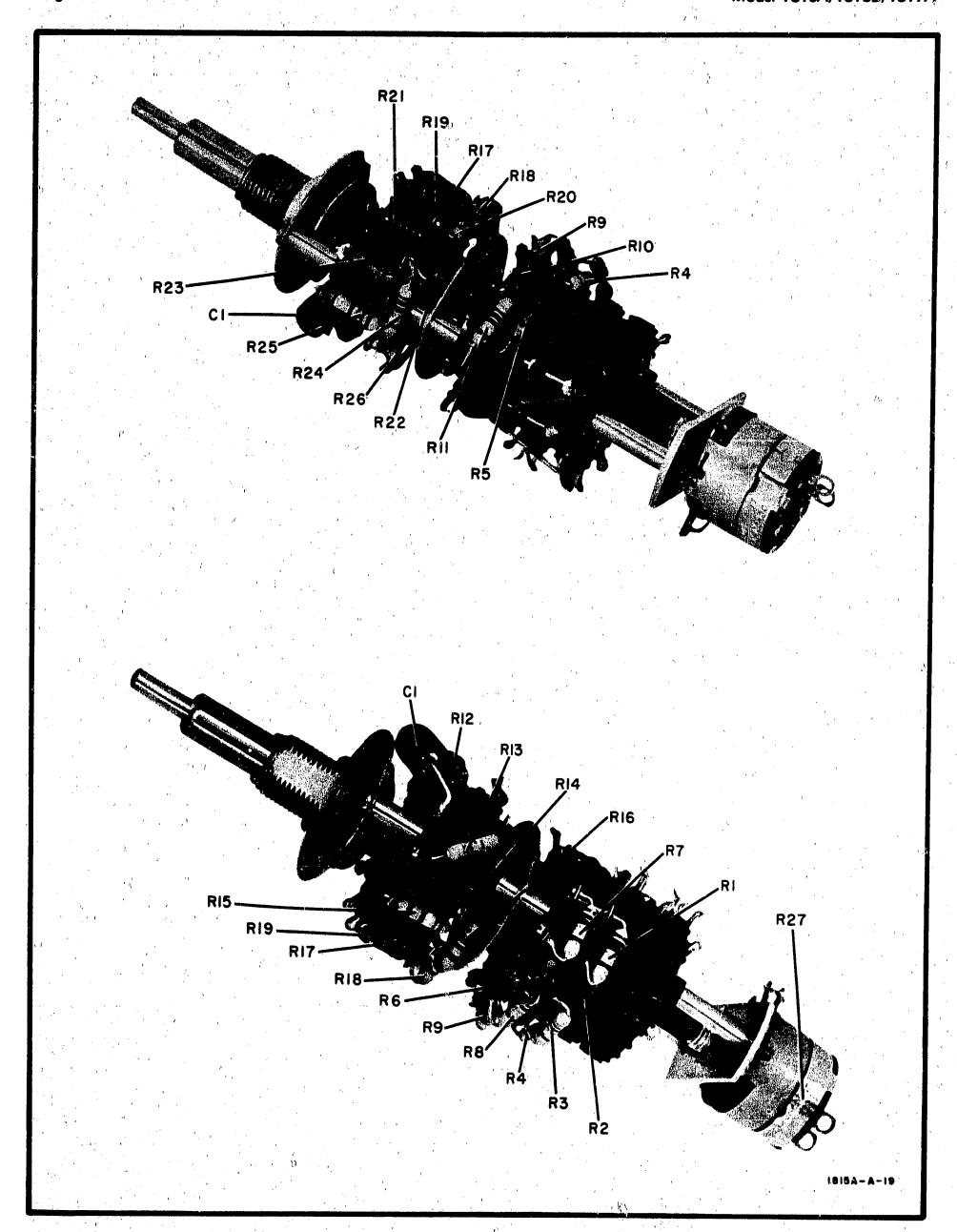
Figure 8-13. p/DIV, VOLTS/DIV Switch Assembly A8 Parts Locations
