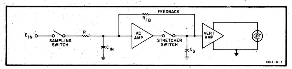
Figure 4-3. Basic Sampler and Vertical Amplifier
