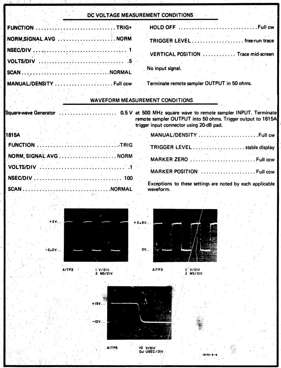
Figure 8-11. Stretcher, Vertical Amplifier Measurements
