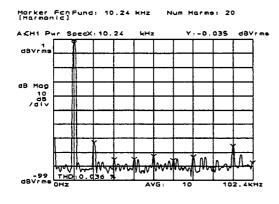
This turns on the harmonic distortion marker and sets the fundamental frequency to equal the current marker position—in this case, 10.24 kHz.
