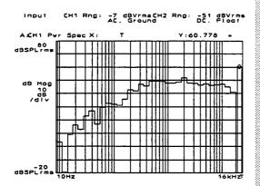
This turns on the analyzer's channel 1 input A-weight filter. Notice how the **AW1** indicator (at the top of the display) turns on—this lets you know that the measurement is now A-weighted.
