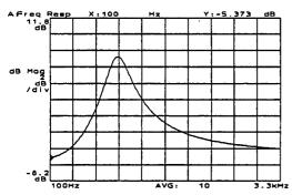
In this example, we used a simple 1 kHz bandpass filter with an adjustable response. Your filter should have an adjustment to vary the bandpass response, though this isn't absolutely necessary.
