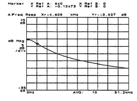
This moves the marker to the largest part of the frequency response trace. Because we are looking at a frequency response trace, the X-marker indicates amplitude in relative terms (dB).
