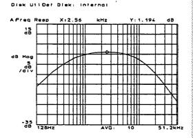
In this example, we're using the analyzer's internal A-weight filter. The choice of a linear or logarithmic X-axis is not critical—math operations are not affected by this decision.
