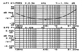
Note how the product of the inverse trace and the orignal frequency response trace is a flat line.
