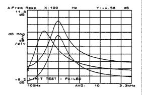
In the first example, we changed the peak response of the test filter. In the second example, we changed the center frequency of the test filter from 1 kHz to 500 Hz.
