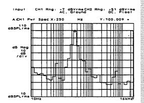
This sets the amplitude of the current marker position to 100 dBspl(rms). Until you change this reference (or preset the analyzer), all amplitude values are referenced to an absolute level of 100 dBspl(rms) if you use engineering units.
