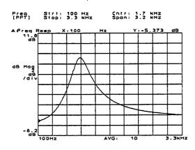
In this example, we used a simple 1 kHz bandpass filter with an adjustable response. Your filter should have an adjustment to vary the bandpass response, though this isn't absolutely necessary.
