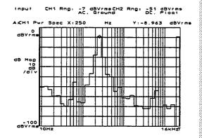
This moves the marker to the 250 Hz third-octave band. The level in this example is about -9dBVrms. For an acoustics measurement, however, we need to set this marker value to 100 dBspl, since we know this to be the absolute level of this microphone calibrator. In a moment, we'll show how to do this with *engineering units*.
