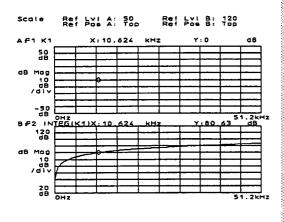
This shows the integrated function. The curve appears to be exponential because the analyzer's default trace coordinate is dB magnitude. This is because in dB magnitude, the Y-axis is logarithmic.
