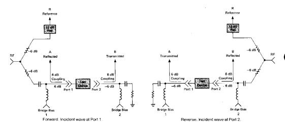
With these connections, the forward (input) and reverse (output) parameters as follows:
