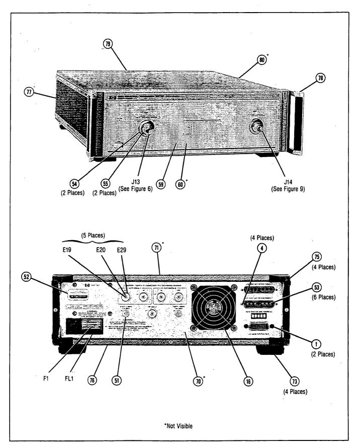
Figure 8. HP 8513A Miscellaneous Mechanical, Chassis, and Electrical Parts (1 of 5)
