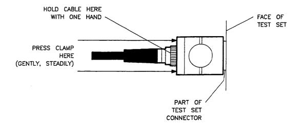
Figure 12. Mating the Clamp and Nut Flats
