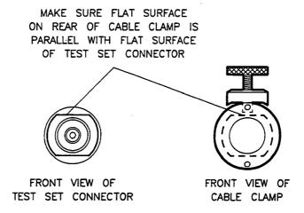
Figure 11. Visually Aligning Clamp and Nut Flats
