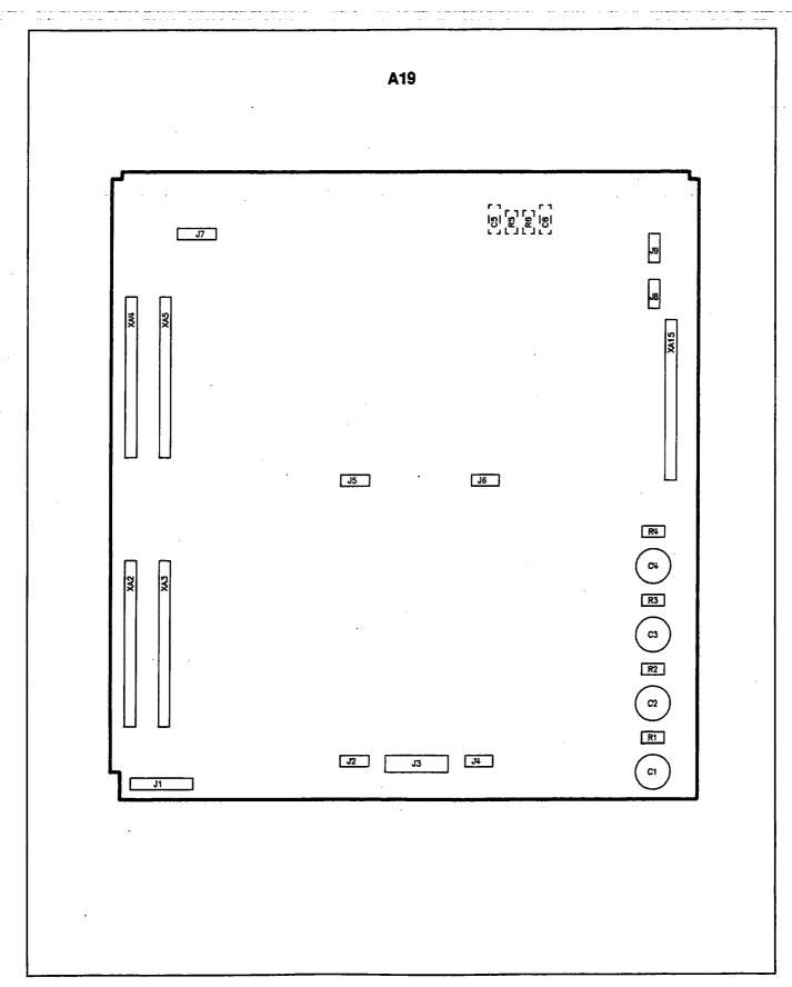
Figure 5. HP 8515A and A513A Motherboard Component Location Diagram
