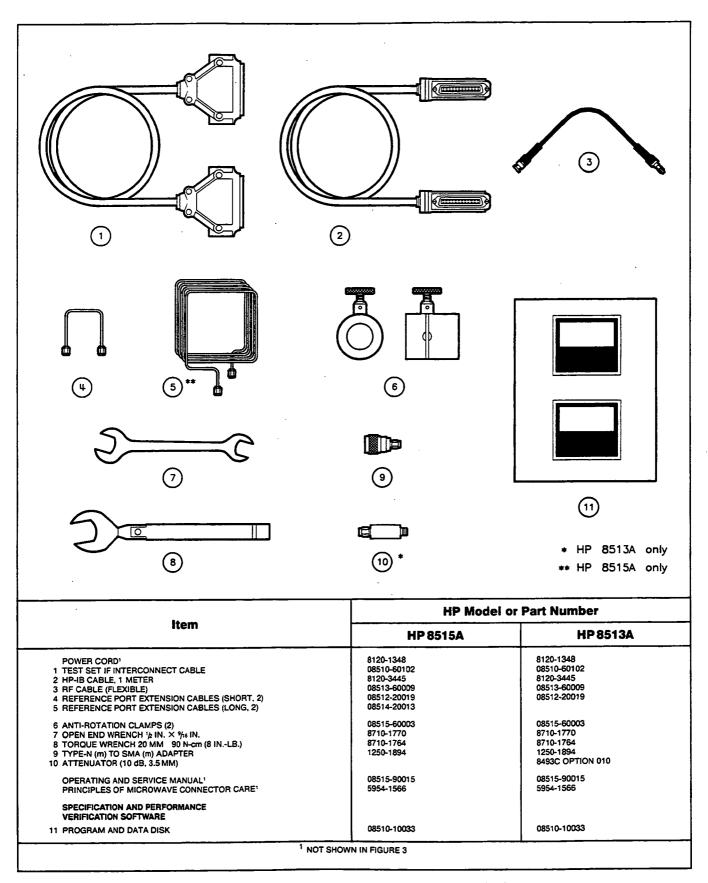
Figure 3. Accessories supplied with HP 8515A and HP 8513A
