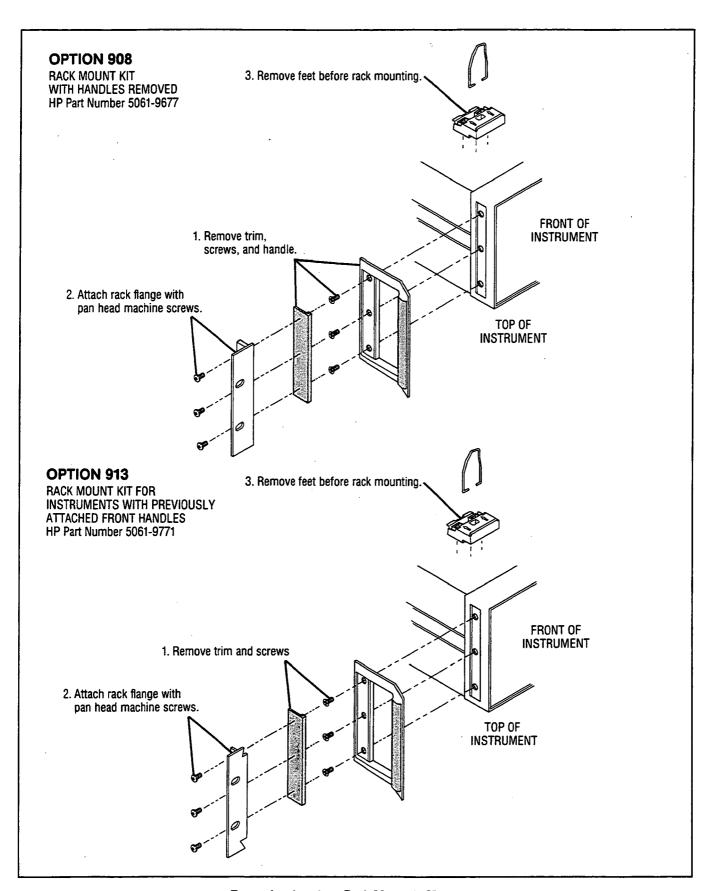
Figure 4. Attaching Rack Mounting Hardware
