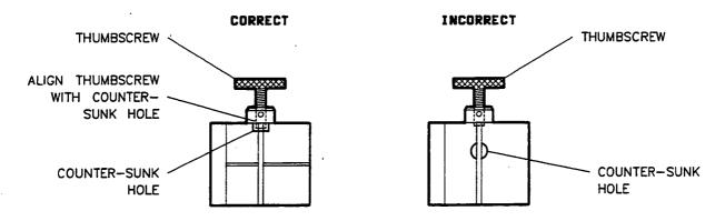
Figure 13. Aligning the Thumbscrew with the Counter-bored Hole
