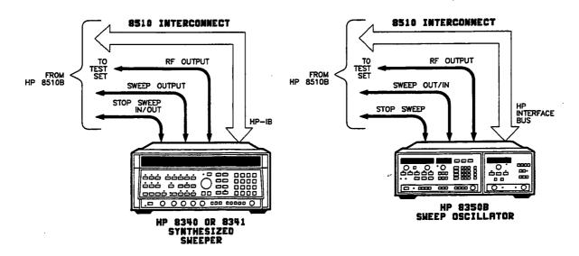
Figure 5. HP8515A and 8513A System Connections
