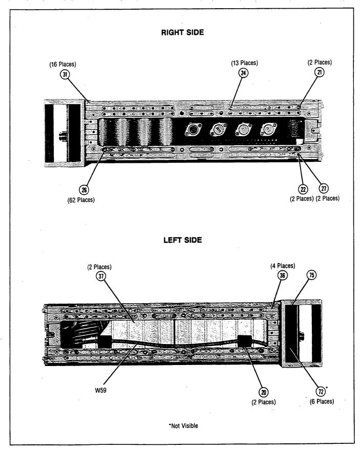
Figure 2. HP 8515A Miscellaneous Mechanical, Chassis, and Electrical Parts (2 of 5)
