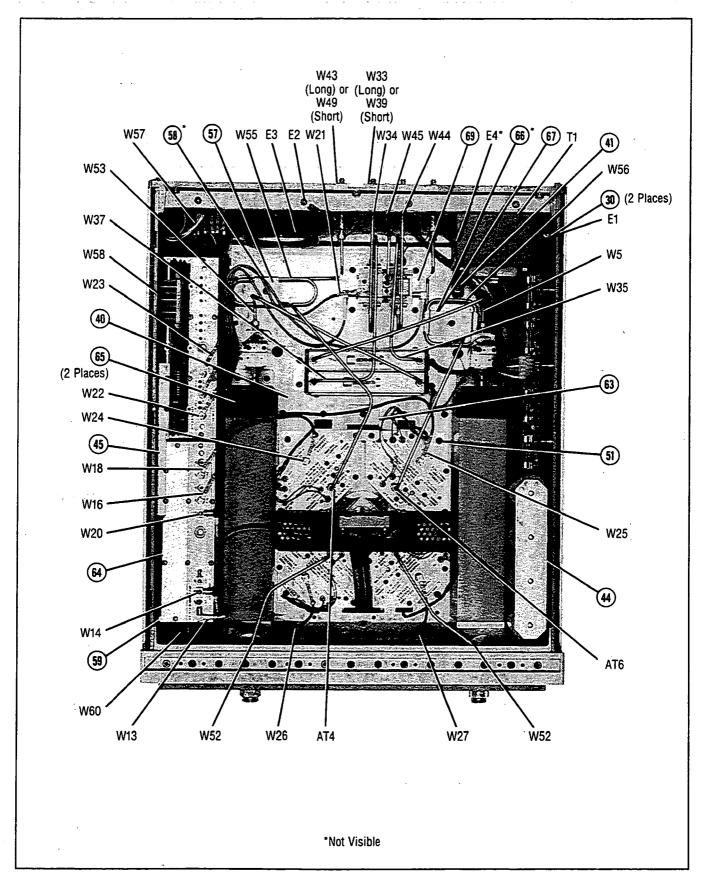
Figure 2. HP 8515A Miscellaneous Mechanical, Chassis, and Electrical Parts (4 of 5)
