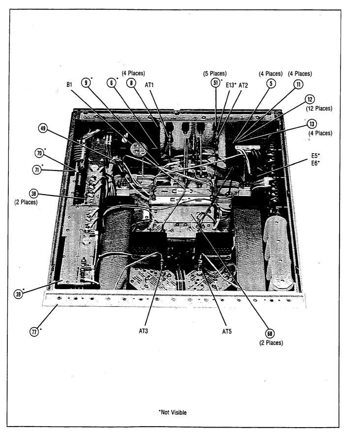
Figure 2. HP 8515A Miscellaneous Mechanical, Chassis, and Electrical Parts (5 of 5)
