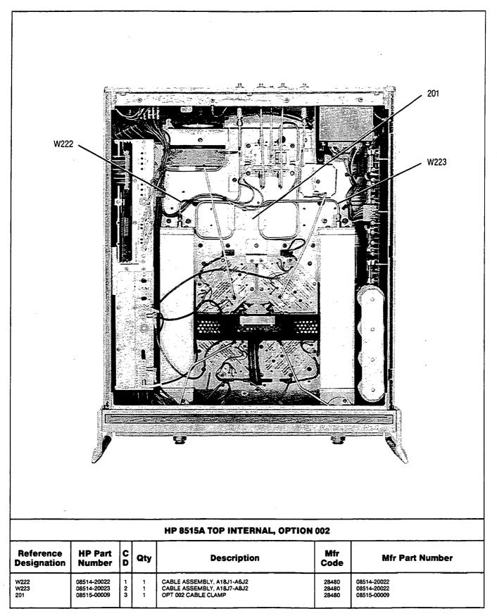
Figure 4. Parts Unique to HP 8515A Option 002
