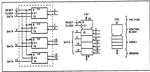
Figure 8-10. Common Control Block
