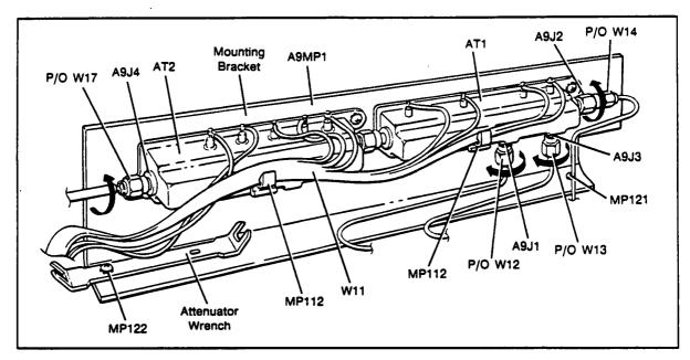
Attenuator Assembly A9 (2425A and above)
