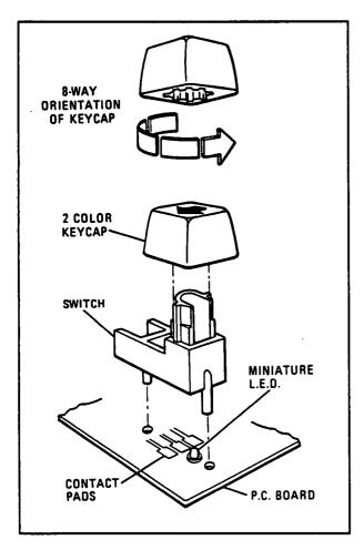
Figure 8-3. Front-Panel Pushbutton Switch Assembly
