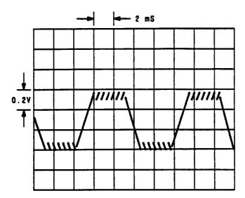
Figure 6. Oscilloscope Display of TP3 (dc coupled), Signal Generator's frequency 950 MHz, modulation EXT FM 5 kHz deviation (100 Hz square wave).
