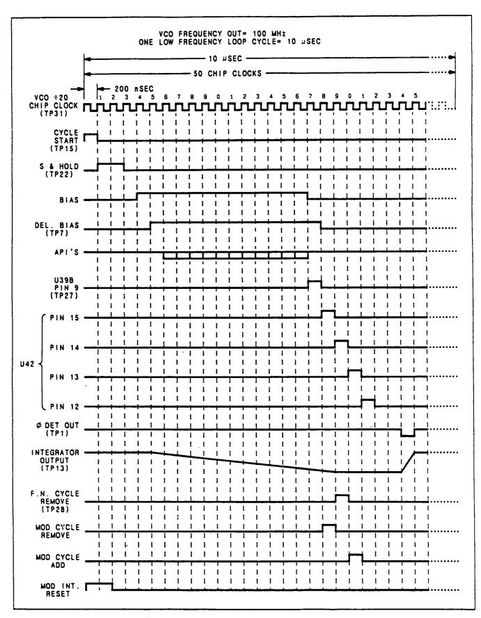
Figure 7. Low Frequency Loop Timing Diagram
