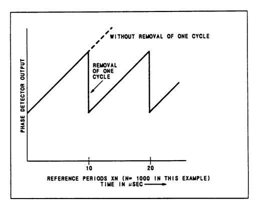
Figure 3. The Output of the Phase Detector Shown. Here is a Sawtooth Riding on a dc Voltage.
