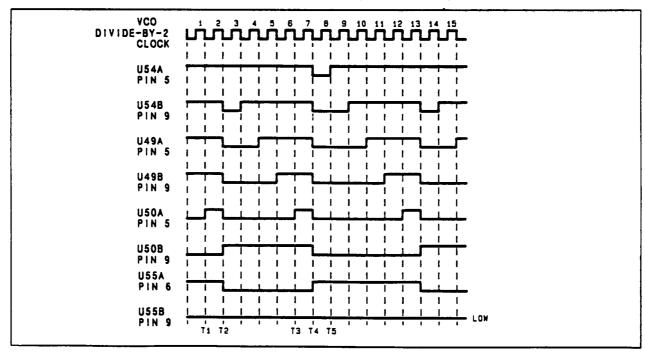
Figure 2. Divide-By-11 Timing Diagram
