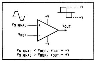
Figure 8-23. Non-Inverting Comparator
