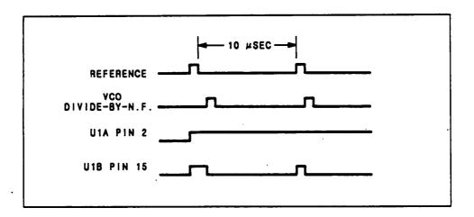
Figure 2. Timing Reference Leads VCO Divide-By-N.F.
