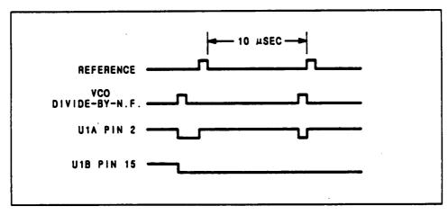
Figure 1. Timing VCO Divide-By-N.F. Leads Reference
