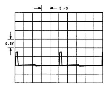
Figure 4. Oscilloscope Display of TP12 (dc coupled), W3 in W3A position, Low Frequency Loop locked, Signal Generator's frequency 950 MHz.
