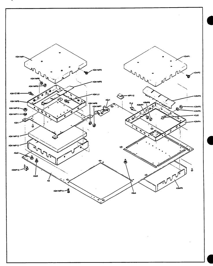
Figure 6-4 (2511A and above). Low Frequency Loop Assembly—A3, Parts Identification
