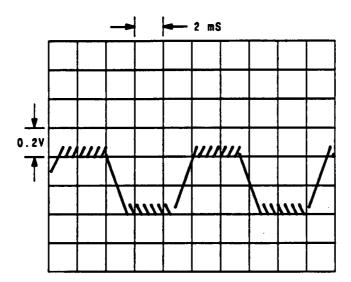
Figure 2. Oscilloscope Display of TP3 (dc coupled), Signal Generator's frequency 950 MHz, modulation EXT FM 5 kHz deviation (100 Hz square wave).
