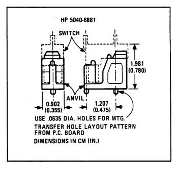
Figure 8-4. Pushbutton Switch Support Anvil
