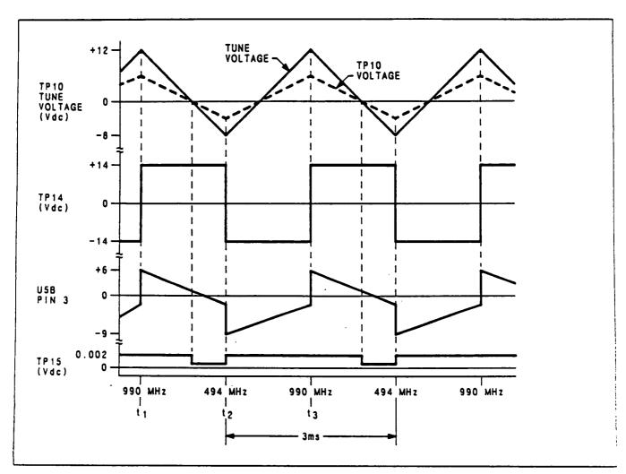
Figure 1. Unlocked High Frequency Loop Waveforms
