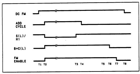
Figure 1. FM Calibration Timing Diagram
