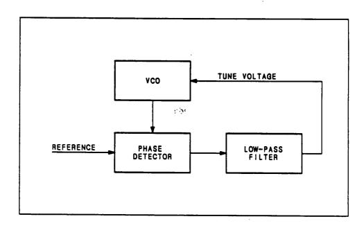
Figure 1. Basic Single Frequency Phase Lock Loop
