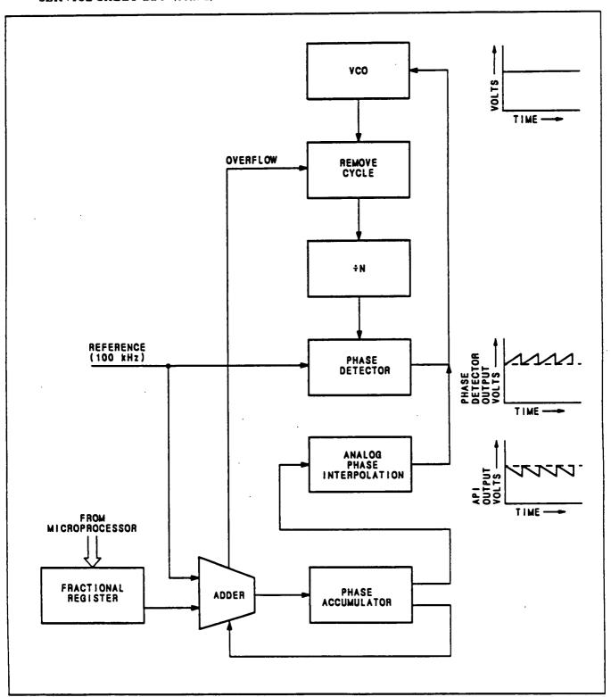
Figure 7. Simplified Diagram of a Fractional-N Phase Lock Loop
