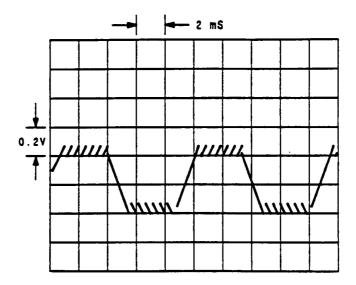
Figure 9. Oscilloscope Display of TP3 (dc Coupled), Signal Generator's Frequency 950 MHz, Modulation EXT FM 5 kHz Deviation (100 Hz Square Wave)
