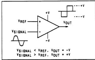
Figure 8-24. Inverting Comparator
