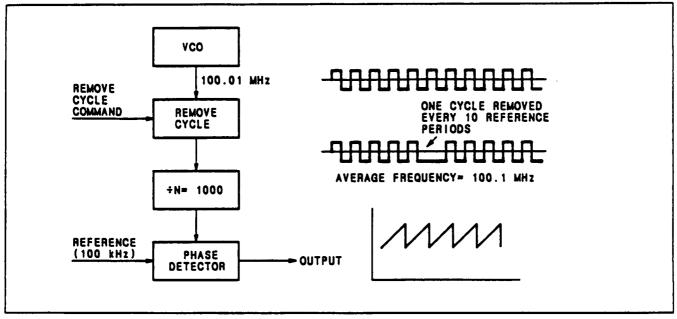
Figure 4. The Basic Block Diagram of a Modified Divide-by-N Loop With a Pulse Remover Added to Allow the VCO to Operate at a Fractional Frequency
