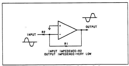
Figure 8-22. Inverting Amplifier (Gain = -R1/R2)
