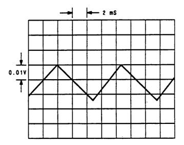
Figure 3. Oscilloscope Display of TP4 (dc coupled), Signal Generator's frequency 950 MHz, modulation EXT FM 99 kHz deviation (100 Hz square wave).
