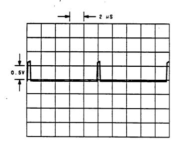
Figure 9. Oscilloscope Display of TP11 (dc coupled), W3 in position W3B (service position), Signal Generator's frequency 950 MHz.
