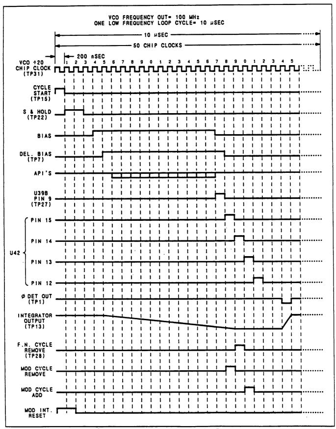
Figure 8. Low Frequency Loop Timing Diagram
