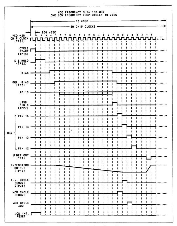
Figure 1. Low Frequency Loop Timing Diagram
