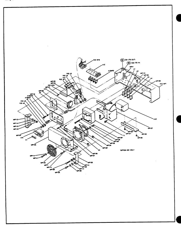
Figure 6-3 (2425A to 2509A). Rear-Panel, Parts Identification
