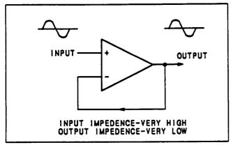
Figure 8-20. Non-Inverting Amplifier (Gain = 1)
