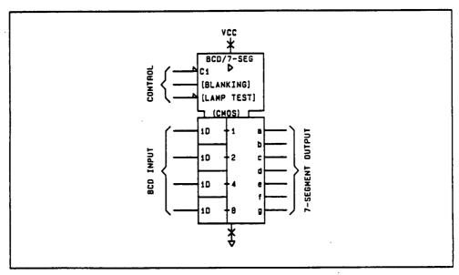
Figure 8-19. BDC-to-Seven-Segment Latch/Decoder/Driver
