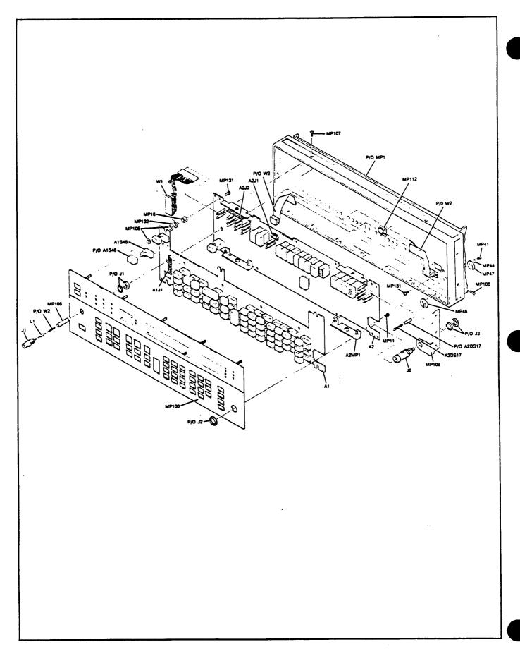
Figure 6-2 (2511A and above). Front-Panel, Parts Identification
