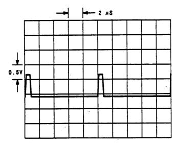
Figure 6. Oscilloscope Display of TP12 (dc coupled), W3 in W3A position, Low Frequency Loop locked, Signal Generator's frequency 990 MHz.
