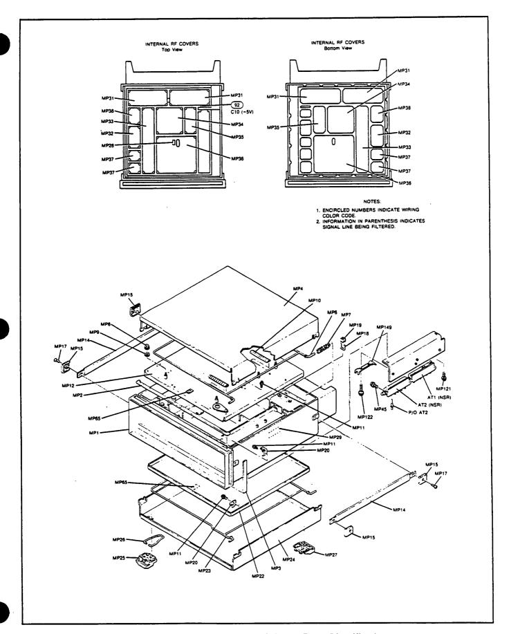
Figure 6-1 (2511A and above). Cabinet, Parts Identification
