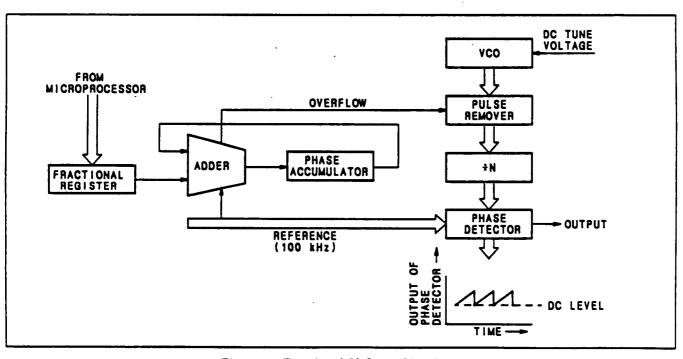
Figure 5. Fractional-N Loop Showing a Phase Register Used to Trigger the Removal of one VCO Cycle (or Pulse)
