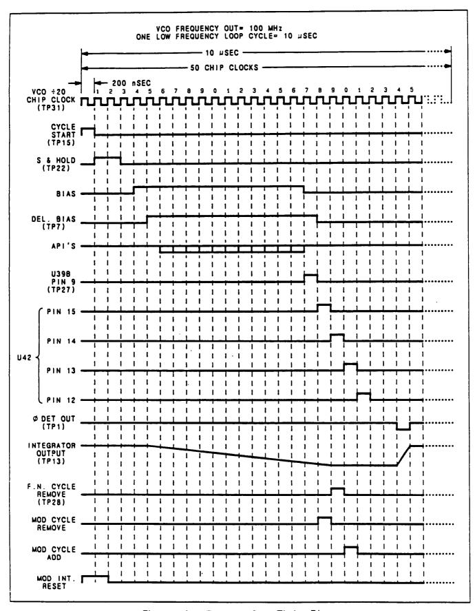
Figure 1. Low Frequency Loop Timing Diagram
