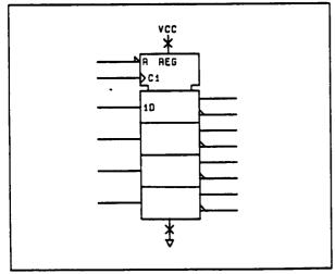
Figure 8-13. Quad D-Type Latch
