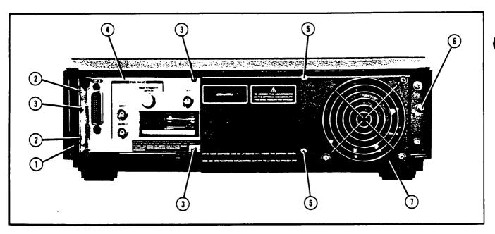
Figure 8-2 (2425A to 2509A). Rear-Panel and Fan Shroud Removal
