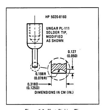
Figure 8-5. Heat Staking Tip
