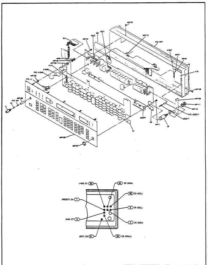
Figure 6-2 (2425A to 2509A). Front-Panel, Parts Identification
