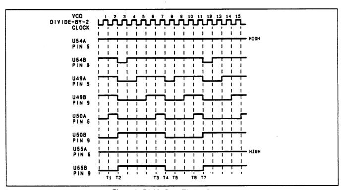
Figure 3. Divide-By-9 Timing Diagram
