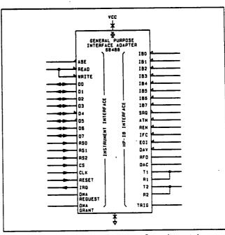
Figure 8-18. General Purpose Interface Adapter
