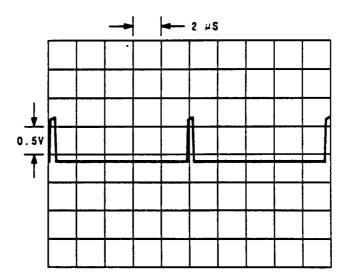
Figure 10. Oscilloscope Display of TP12 (dc coupled), W3 in position W3B (service position), Signal Generator's frequency 950 MHz.
