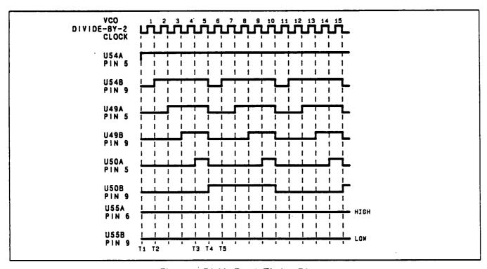
Figure 1. Divide-By-10 Timing Diagram
