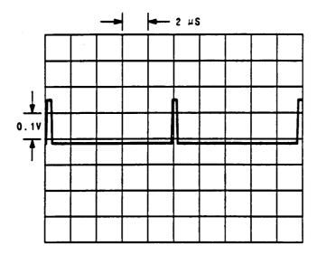
Figure 8. Oscilloscope Display of TP22 (dc coupled), Sample and Hold Pulse, W6 removed, Signal Generator's frequency is 950 MHz, Low Frequency Loop is unlocked.
