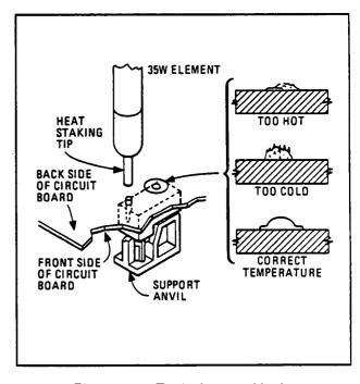
Figure 8-6. Typical Assembly for Heat Staking Operation
