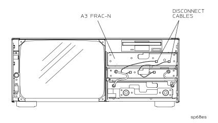
6. Grasp the handle tab and pull forward to release the assembly. Once released, the assembly will easily slide out of its cavity.
