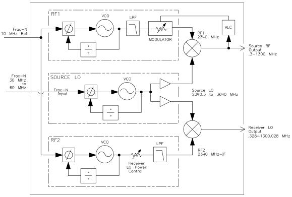
The power level of the Source RF output is controlled by the firmware on the CPU board. The firmware digitally controls the level setting in the ALC/MODULATOR feedback loop. The firmware combines the desired output level with data from Adjustment #104 to determine the level settings for the ALC/MODULATOR feedback loop. (See Chapter 2, "Adjustments," for more details on the adjustment procedure.) The firmware is able to vary the Source RF output level over a range of approximately 10 dB.
