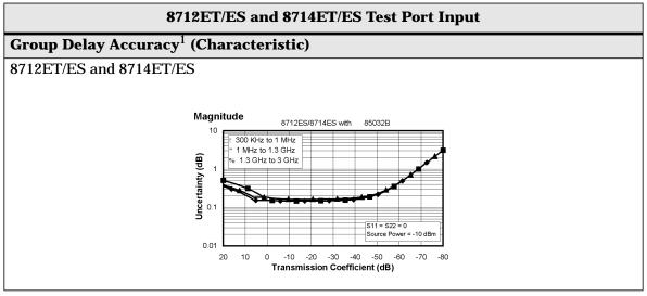
1. Valid for 85032B/E (type-N 50  $\Omega$ ) and 85036B/E (type-N 75  $\Omega$ ) cal kits using either a two-port or enhanced response calibration.
