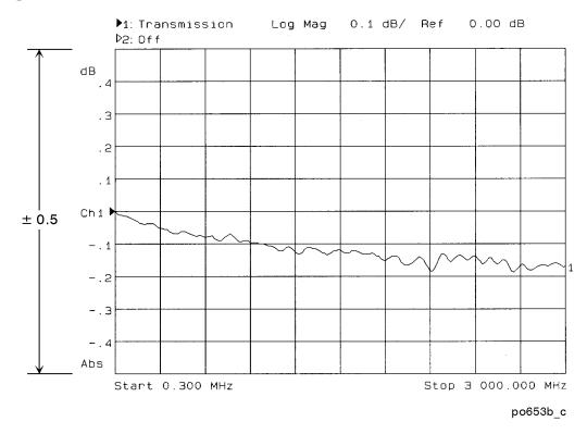
Figure 1-2 Verify Transmission (or  $S_{21}$  and  $S_{12}$ ) Measurement
