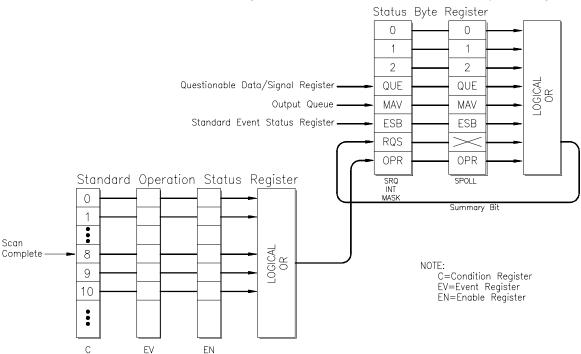
The various registers are set and queried using decimal weighted bit values. The decimal equivalent for bits 0 to 15 is shown below.
