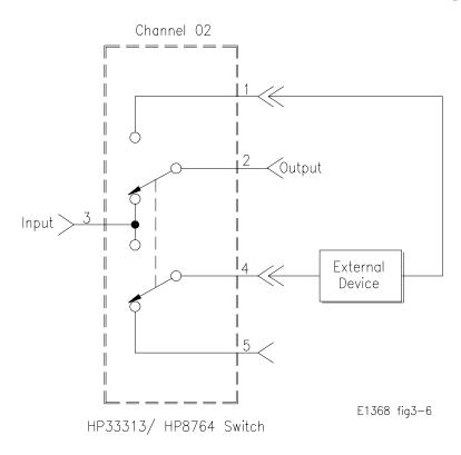
Figure 3-6. Example: Transfer Switch (one channel)
