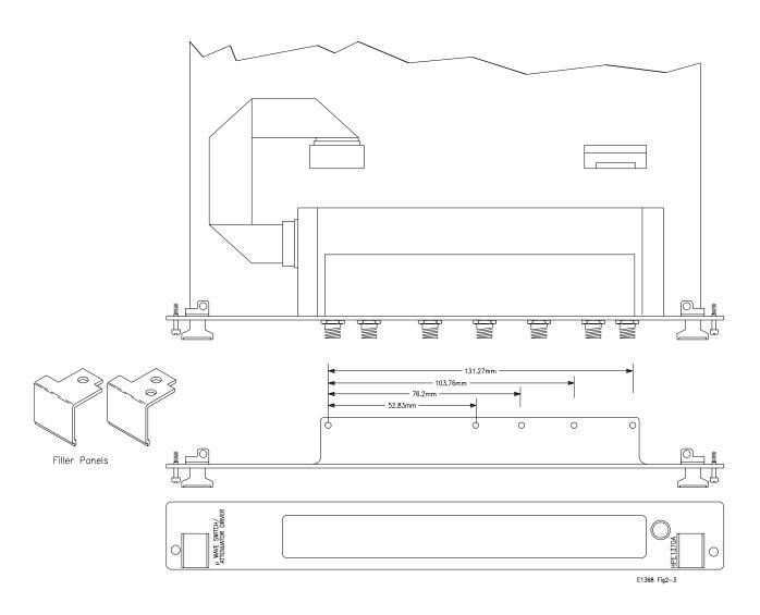
Figure 2-7. Microwave Switch/Attenuator Installation
