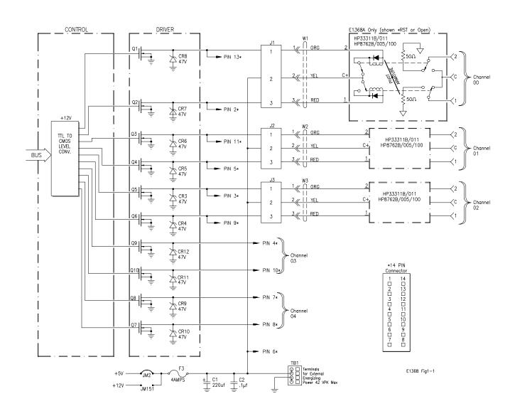
Figure 1-1. HP Microwave Switch Block Diagram
