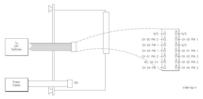
Figure 2-4. Microwave Switch Connection
