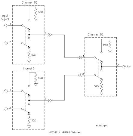
Figure 3-7. Example: 4-Channel Multiplexer
