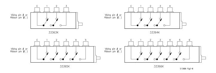
Figure 2-8. Internal Switch Diagrams
