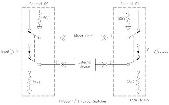
Figure 3-5. Example: Transfer Switch (two channel)
