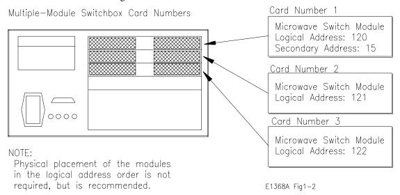
Figure 1-2. Card Numbers for Multiple-Module Switchboxes
