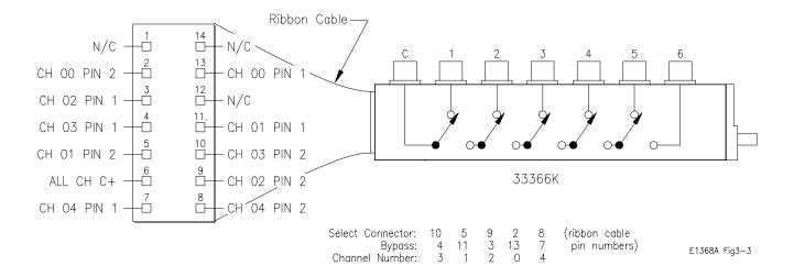
Figure 3-3. Example: HP E1370A Multiple Channel Switching
