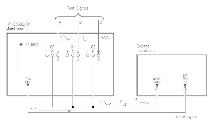
Figure 3-9. Example: Multiple Channel Scanning
