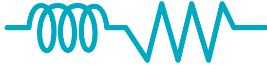
Figure 1. Equivalent circuit of a ferrite bead
