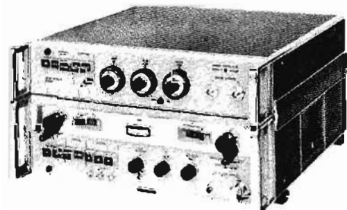
Figure 7. Joining brackets effectively weld instruments into a single physical unit.
