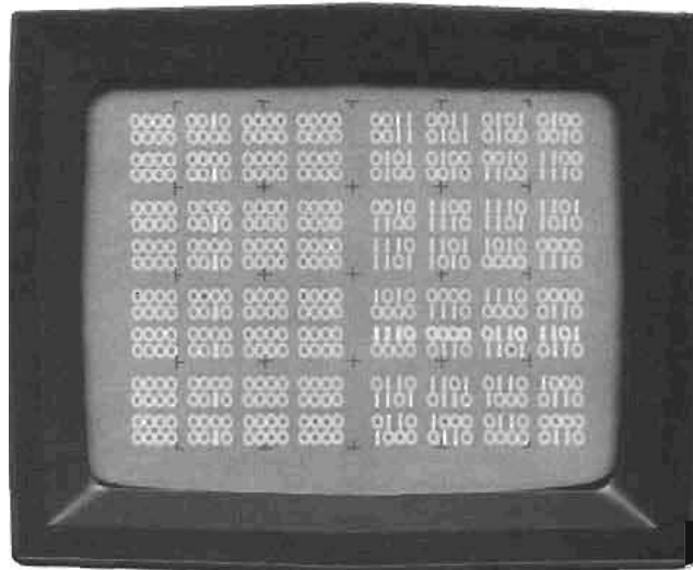
In the exclusive OR mode, A & (A ⊕ B), A memory data is displayed on the left while the table on the right displays logic differences between A and B memories. This provides very fast "at-a-glance" comparisons.
