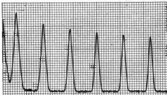
Figure 5a. This represents a portion of a frequency multiplexed system operating normally. Notice that not all channels are operating at the same level.
