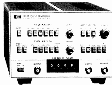
HP 8011A with Option 001, Burst
