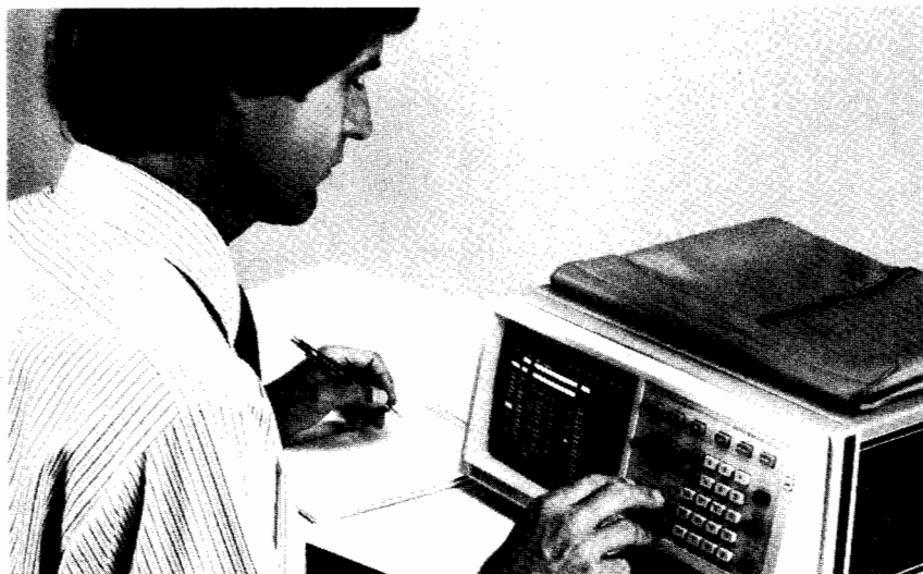
Benchtop logic analyzers provide state, timing and performance analysis for troubleshooting and optimizing digital systems in the laboratory and at remote sites.
