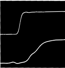
HP 8161A input pulse (upper) and ECL memory output pulse (lower).
