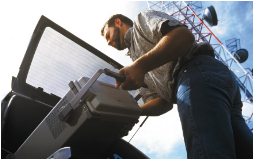
Options allow using the HP 8921A for comprehensive CDPD cell site tests.
