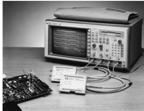
The HP 54542A shown with the HP 1145A, two-channel, 750-MHz, small geometry active probe for surface mount devices.
