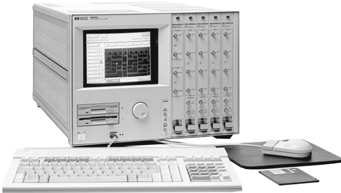
HP 80000 Data Generator System with two strobe and 16 data channels. With the expansion frames, up to 80 channels can be configured.
