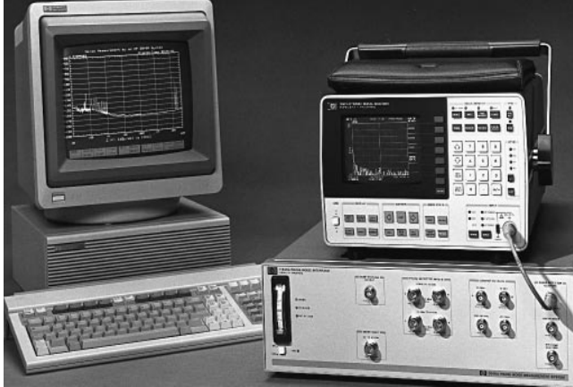
HP 3048AR Phase Noise Measurement System controlled by an HP 98580C desktop computer
