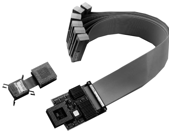
HP's low-profile architecture preprocessors let you connect even when space is limited.
