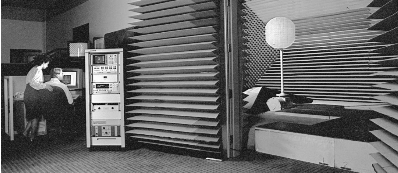
HP 85301B antenna/RCS measurement system in HP's compact test range
