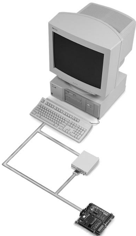
HP Processor Probe with full featured debugger provides a run-control solution.
