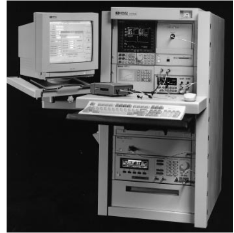
EDFA Test Systems
