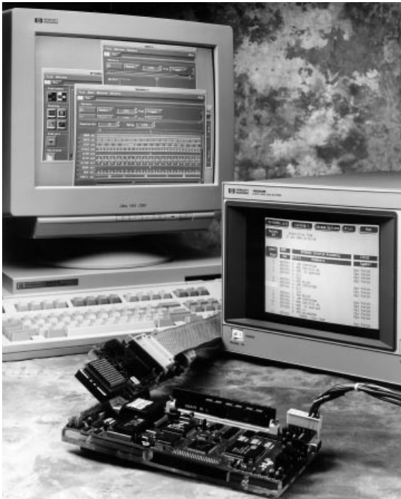
This preprocessor architecture is commonly used for microcontrollers. State, timing, and parametric measurements are available.
