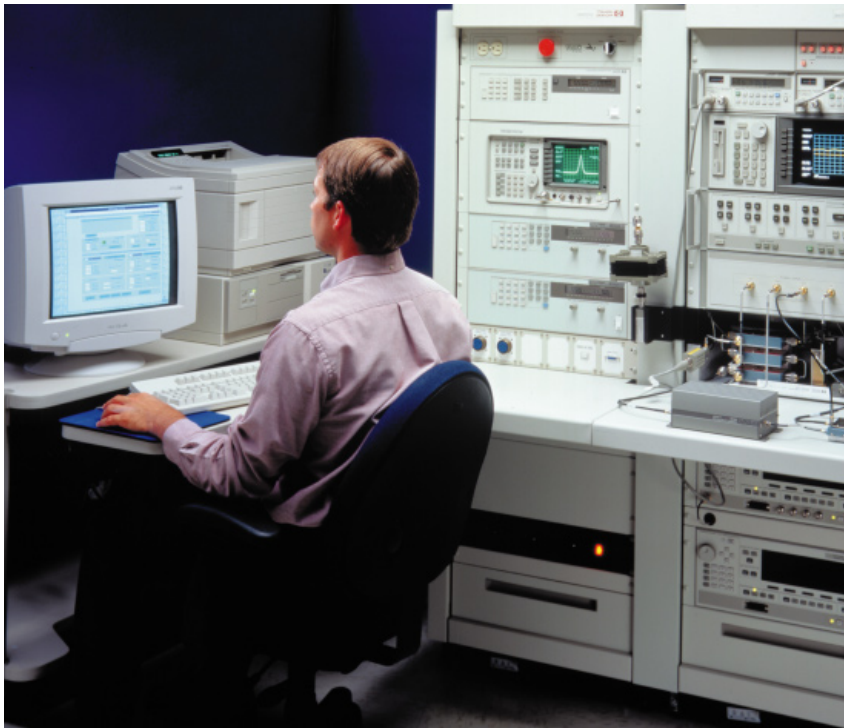
The custom automated HP test system rapidly tests CEL's high-power transistors during development, and facilitates trend analysis.
