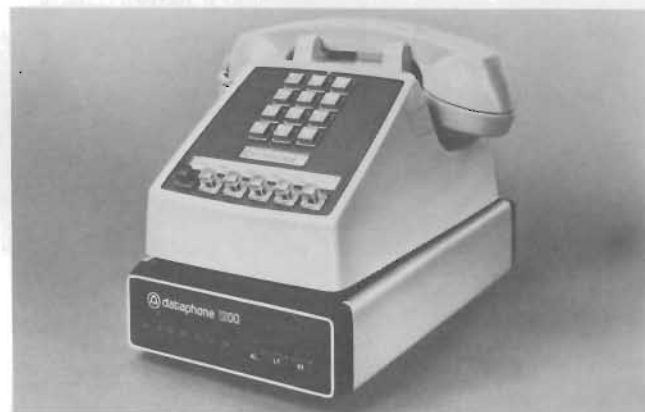
Figure 3-1 Bell 202-Type Data Set (DATAPHONE 1200)
