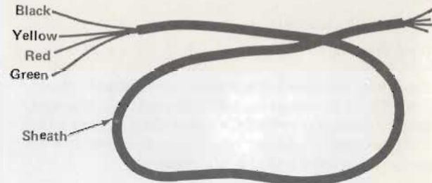
Figure 2-4 Four Wire Line
