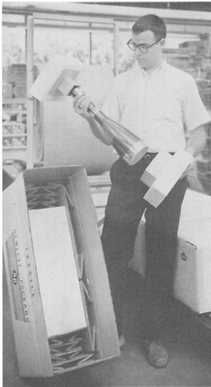
Package being given the "parcel post" test on MEASURE's cover looks like this inside. Bob Holcomb holds cathode ray tube with two special plastic foam and corrugated board end pieces which "float" tube in the single carton. Spring-like corrugated pieces and two cartons (22 pieces) absorb less shock than the 3-piece "floater."
