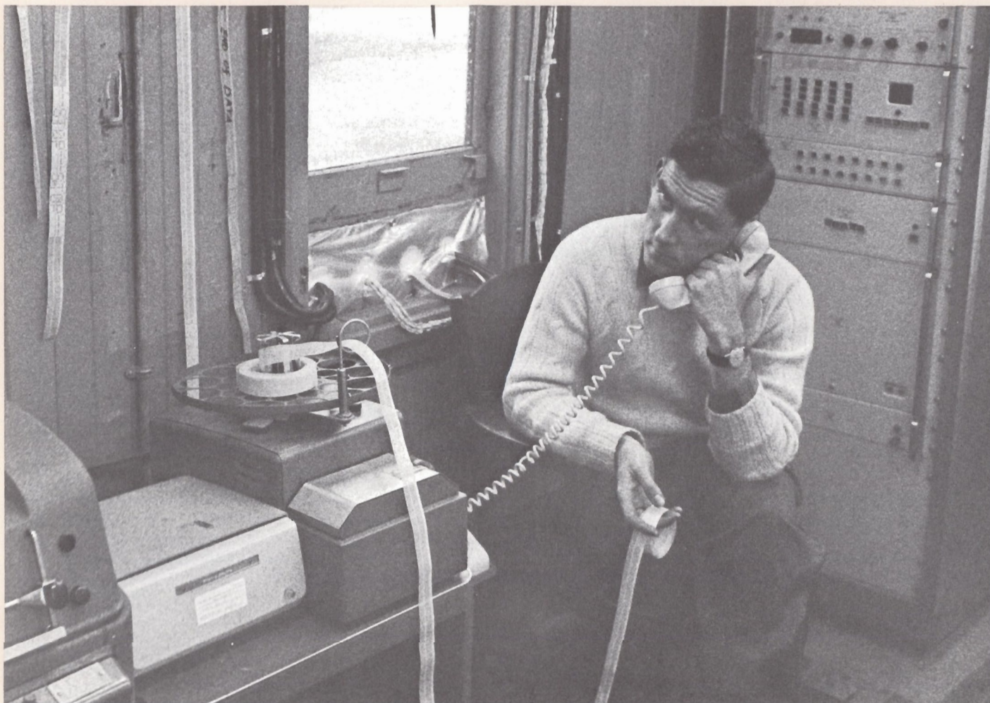
Eight-level tape from the Dymec 2010B system was transmitted 800 miles to Montreal where identical tape was produced and fed into computer.
