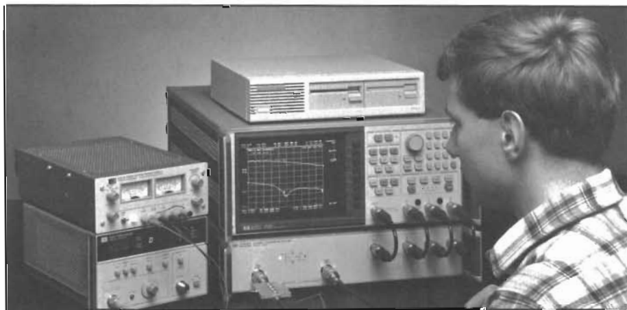
The HP 8753B offers new features for nonlinear measurements and direct control of external instruments.
