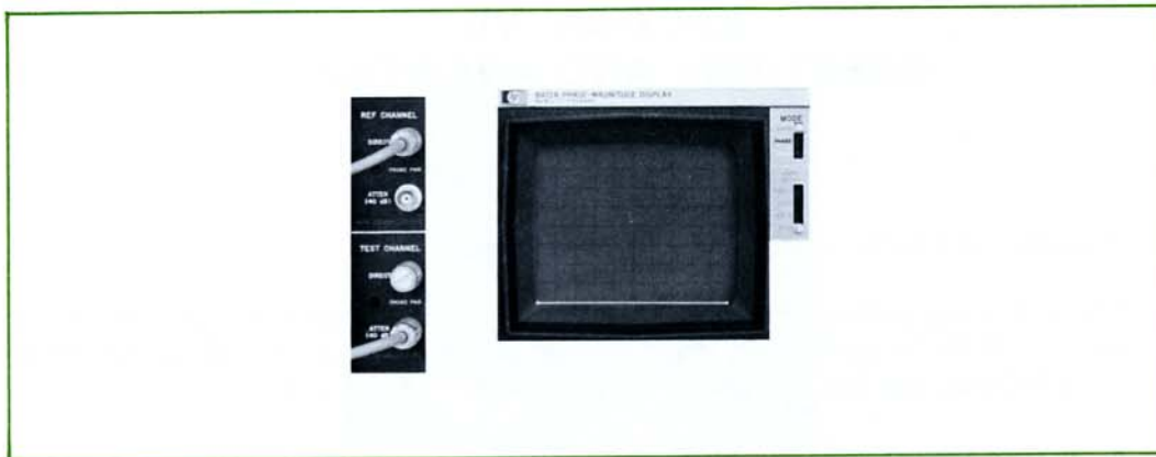
Figure 7-2. Shows how trace should line up with bottom graticule if LOW LEVEL AMPL is adjusted properly.
