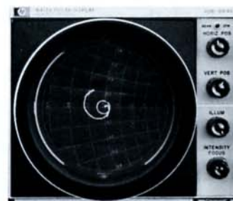
EXAMPLE OF SMITH CHART PLOT OF IMPEDANCE
