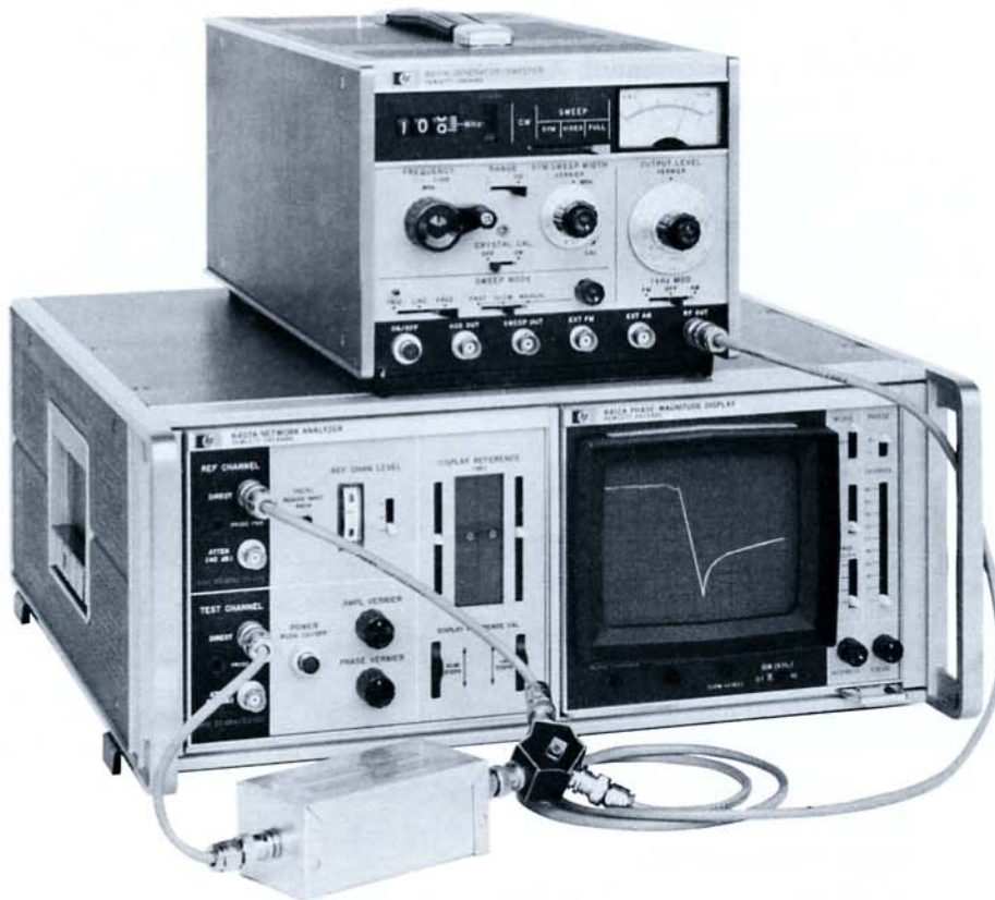
Transmission Measurement of a Low Pass Filter Using the HP 8407A Network Analyzer, 8412A Phase-Magnitude Display, 11652A Reflection-Transmission Kit and 8601A Generator/Sweeper.
