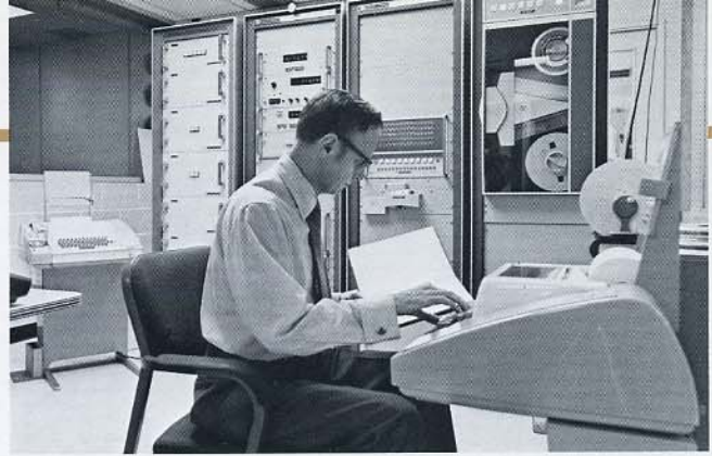
Figure 2. Seated at a teleprinter in the computer room, the operator is entering changes into the process control system by calling the variable number assigned to the particular function, and inserting the new figure. In between printouts, the computer handles non-process jobs via the teleprinter in the rear.
