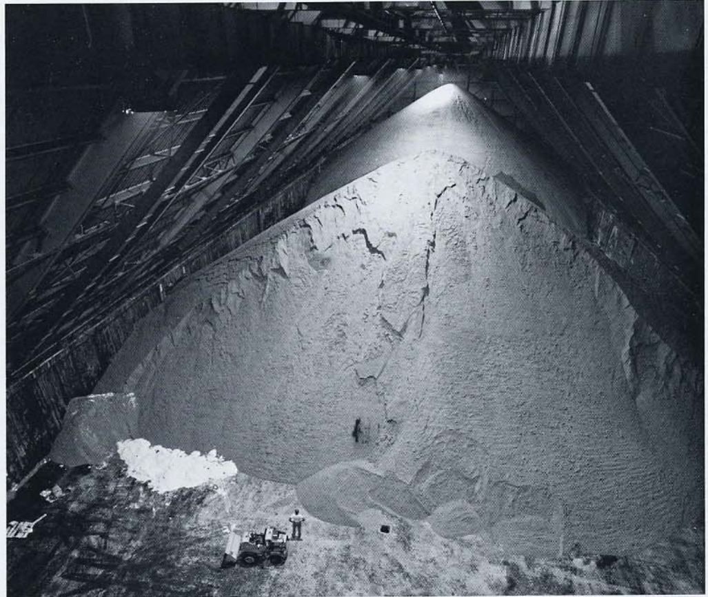
Figure 1. A mountain of raw sugar just waiting to be processed. Redpath's Toronto refinery processes 78,000 pounds per hour.
