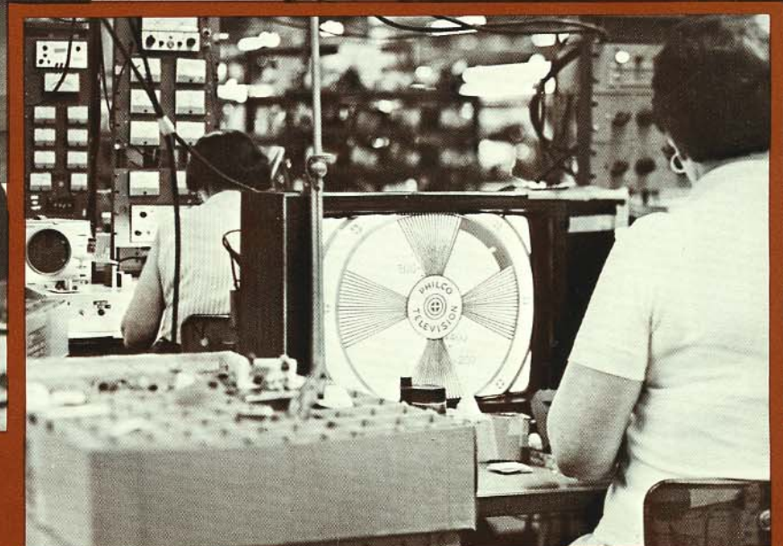
Philco Color TV Modules are aligned and checked by automatic handler and HP 9500 Series System.
