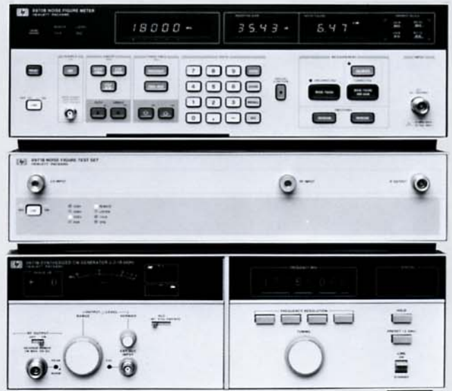
HP 8970T Noise Figure Measurement System (10 MHz to 18 GHz).
