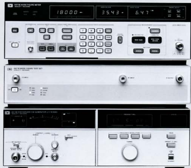
The HP 8971B Noise Figure Test Set (middle instrument) uses a temperature-compensated YIG-tuned filter to make single-sideband measurements. In the HP 8970T system configuration pictured here, the HP 8970B Noise Figure Meter (top) acts as the controller for both the HP 8971B and HP 8671B Synthesized CW Generator (bottom).
