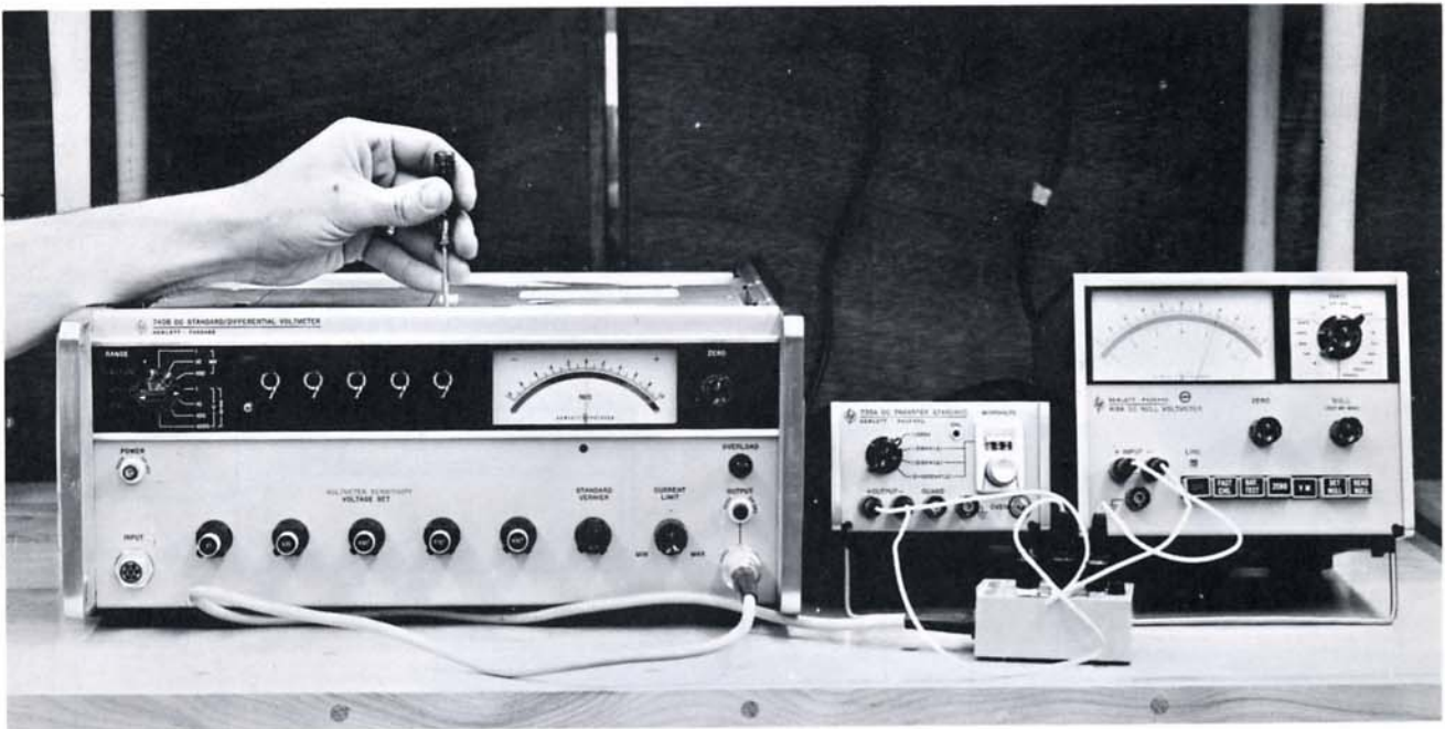
Figure 5-6 Calibration of the Full-Scale Voltage Level of a dc voltage standard.
