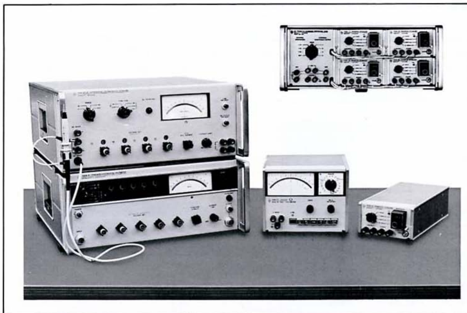
FIGURE 4. Hewlett-Packard's Calibration Standards and Transfer Standards. On the left are the 741B and 740B Calibration Standards; on the right is the 735A Transfer Standard and behind it is the E02-735A Transfer Standard; the nullmeter in the middle is the Model 419A.
