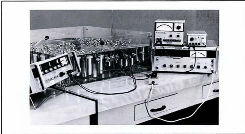
FIGURE 13. The Calibration System Showing the Divider Resistors in an Oil Bath.
