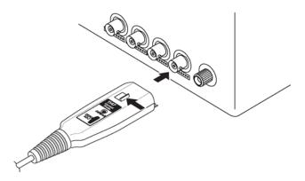
Figure 3. Connecting the Probe to the Oscilloscope
