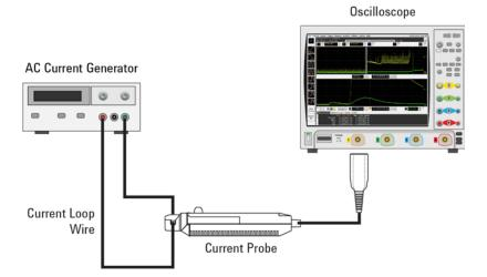
Figure 6. Sensor Head Clamped to Wire
