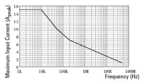
Figure 8. Derating According to Frequency
