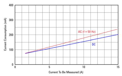
Figure 1. Typical Probe Consumption
