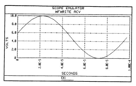
Example 2: Adding a Phase Shift to a Special Function Sine Wave
