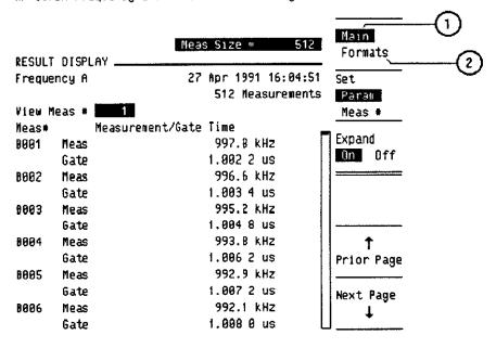
The Numeric display shows the individual measurements that are plotted on the TVar display.
