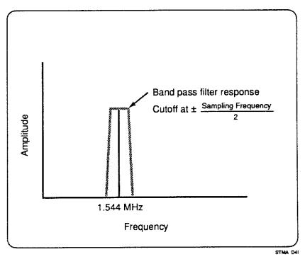
Unfortunately, it is very difficult to construct a good frequency-selectable, band-pass filter. This means that you must be very careful when measuring signals. A good rule is to suspect every spur and test for aliasing by changing the sample rate and watching for spurs changing frequency. (This is demonstrated in chapter 2, "Step three. Check for aliased components in your FFT graph.")
