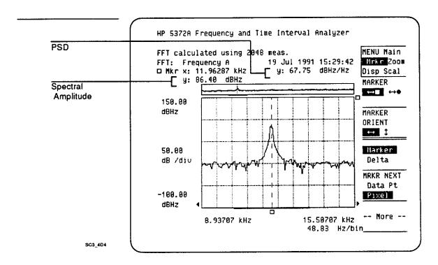
The PSD value is not provided directly over the HP-IB. To determine the PSD value over the bus, you would send the "PSDS?" query to return the power spectral density conversion factor. This value is to be subtracted from the original FFT results. In this example you would receive a value of 18.65. This value could then be used to convert the non-spur value to the PSD value. The same conversion factor applies to the entire FFT acquisition.
