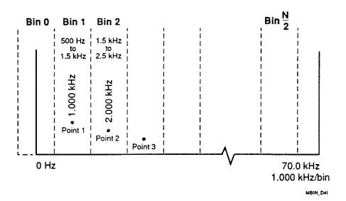
For a case where the frequency bin width is 1.000 kHz/bin:
