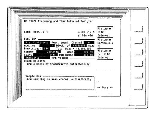
The Histogram measurements are similar to time interval measurements in the way data is collected. The differences are the rate at which data is collected and in how the data is processed and displayed.
