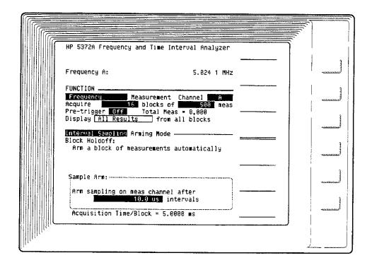
When the number of blocks is set greater than one, it is possible that not all measurements will fit into measurement memory. *Figure 7-3* shows an example where a multiple block measurement does fit in memory. The following results features are available for the menu shown in *Figure 7-3*:
