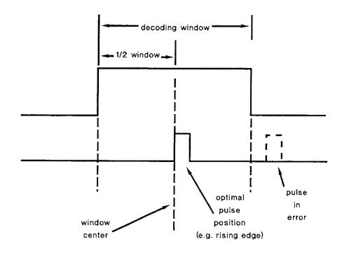
In general, the location of data pulses relative to the decoding window will have some distribution. *Figure 4-19* shows that the distribution can be characterized by two effects: a displacement from the center of the window corresponding to aggregate timing offsets (static bit shift), and a width or sigma, corresponding to the random bit shift effects or aggregate timing "noise". The error rate of the system can be described by the area of the distribution truncated by the decoding window.
