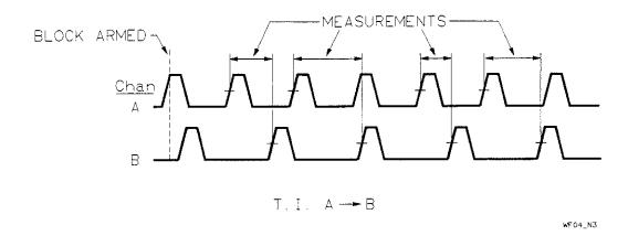
Figure 1-17. Time Interval | Automatic
