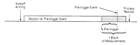
For a single block, continuous monitoring of measurement results occurs until the Pre-trigger condition is satisfied.
