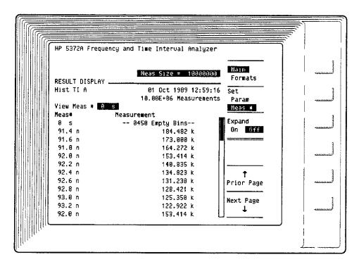
Figure 4-17. Numeric Results of Histogram Measurement, Last Page
