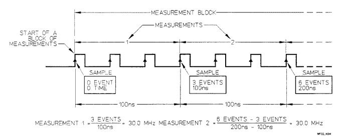
Figure 2-2. Trigger Events Occurring Faster than They can be Stored
