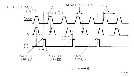
Figure 5-28. REPETITIVE EDGE Timing Diagram
