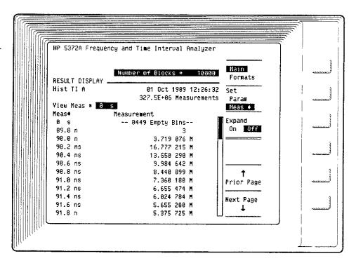
In situations where there is a possibility of over 16 million measurements landing in one bin, use the increased bin height selection AND set the number of measurements per block to less than 16,777,215. Figure 4-5 shows an example of a setup where bins would not overflow. There will be no overflow because at the end of each block of measurements, the bins are cleared and the accumulated counts are stored in software. This processing does slow the rate of data acquisition.
