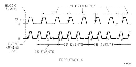
Figure 2-12. Frequency | Cycle Sampling
