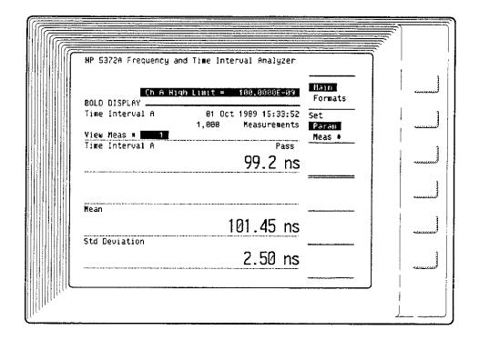
The Bold Display is convenient for viewing measurement results from a short distance away. A result from each measurement acquisition is displayed. If Statistics is enabled, the mean and standard deviation for all measurement data are shown as well. If Limits are enabled, the limit status for the displayed measurement is also shown.
