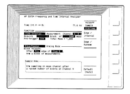
MEASUREMENT: Time Interval, ± Time Interval (two-channel)
