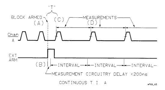
Figure 5-34. EDGE/INTERVAL Timing Diagram
