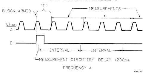
Figure 2-14. Frequency | Edge/Interval DESCRIPTION OF DIAGRAM:
