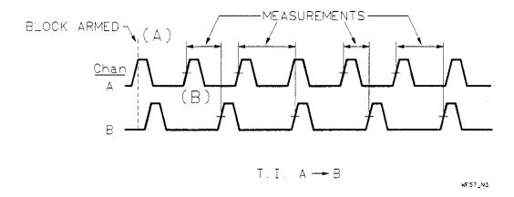
Figure 5-10. AUTOMATIC Timing Diagram
