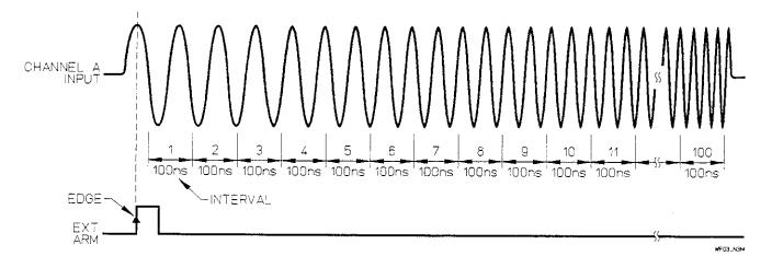
Figure 5-4. Edge/Interval Arming Example
