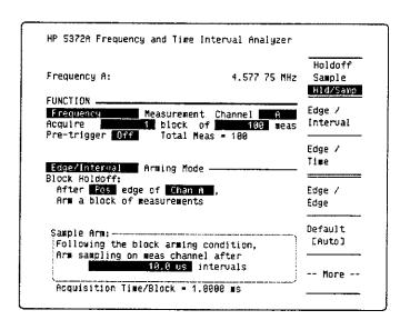
Measurements are acquired in a group. The group of measurements is called a "block." For example, 1 block of 100 measurements. The HP 5372A will make 100 measurements without stopping. This is an example of a continuous arming process.
