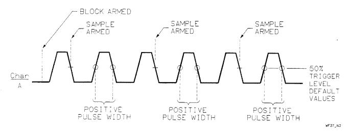
Figure 3-10. Positive Pulse Width A
