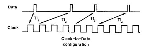
The HP 5372A lets you select the polarity of data edges and clock edges. The setup shown in *Figure 4-22* is recommended for data-to-clock measurements. In this example, the time interval measurement is configured to start on a positive edge of channel A (data) and stop on a positive edge of channel B (clock). The resulting histogram distribution will then be centered about a time interval value equal to the window width.
