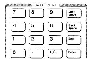
Data Entry keys are used to enter numbers into the numeric fields of the menu screens.
