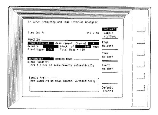
The arming mode is Automatic. Automatic arming begins the group of measurements as soon as possible and provides for acquisition of measurement samples as quickly as possible.
