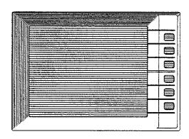
The display and softkey section contains the CRT (cathode ray tube) and the six softkeys. The CRT is a raster-scan, green phosphor display. The screen display resolution is 408 pixels horizontally by 304 pixels vertically. Graph display resolution is 250 pixels horizontally by 180 pixels vertically. The softkeys select the options that appear along the right edge of the display.
