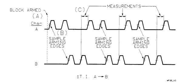
Figure 5-26. PARITY SAMPLING Timing Diagram
