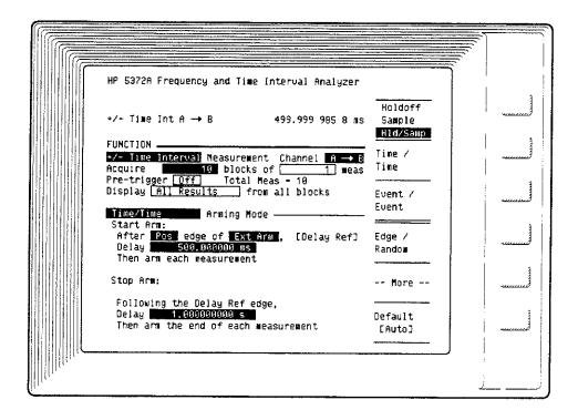
MEASUREMENTS: ± Time Interval, Frequency, and Period
