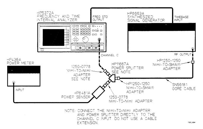
Figure 17-18. Channel C Test Setup
