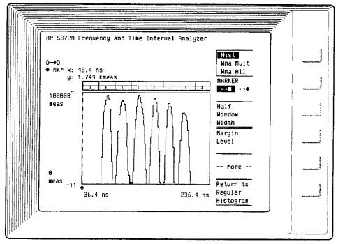
WINDOW MARGIN ANALYSIS MULTIPLE DISTRIBUTIONS (Wma Mult) Early and late window margin information can be retrieved for each of the multiple distributions that can result from data-to-data measurements. The number of distributions will depend on the data pattern; if a constant frequency pattern is measured, the resulting analysis will be the same as the Wma All case.
