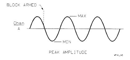
Figure 3-14. Peak Amplitude A
