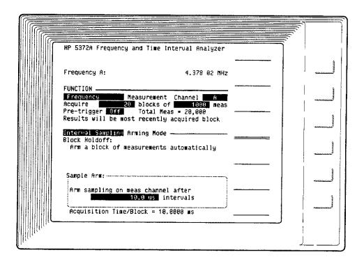
With the number of blocks set greater than one, and the number of measurements per block set so the total number of measurements exceeds the size of measurement memory, the following line of text will appear on the Function menu, "Results will be most recently acquired block." Figure 7-4 shows an example of this situation. The following results are available for the menu shown in Figure 7-4:
