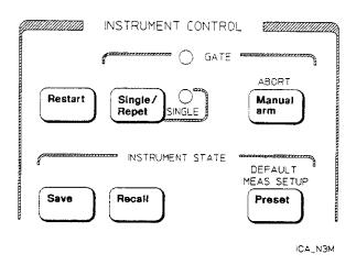
The Instrument Control keys provide control of data acquisition, the Save/Recall registers, and the default setup of the HP 5372A.
