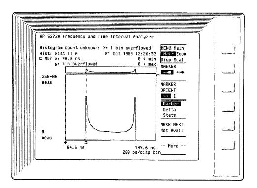
Figure 4-4 shows the Numeric results summary for the Histogram measurement. The bin that overflowed shows a count of 16,777,215 measurements.
