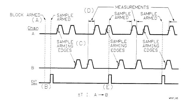
Figure 5-30. REPETITIVE EDGE-PARITY Timing Diagram
