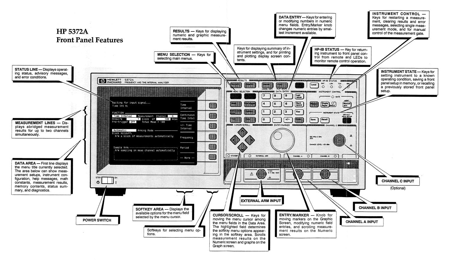
Figure 6-1. Front Panel Features
