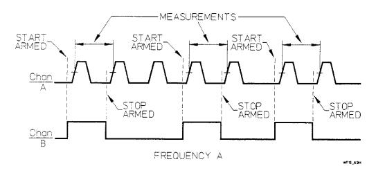
Figure 2-23. Frequency | Externally Gated
