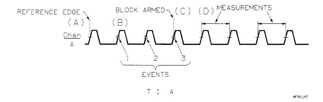
Figure 5-16. EVENT HOLDOFF Timing Diagram
