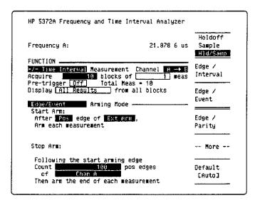
The use of the two terms, "Start Arm and Stop Arm," is intended to communicate that the measurements are collected individually. Each measurement has a start condition and a stop condition. This is non-continuous arming.
