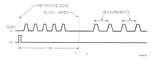
Figure 1-19. Time Interval | Time Holdoff
