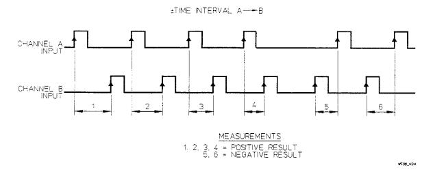
Figure 1-7. ±Time Interval on Two Channels
