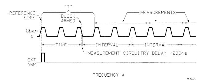
Figure 2-19. Frequency | Time/Interval
