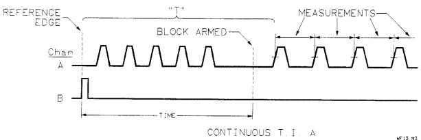
Figure 1-28. Continuous Time Interval | Time Holdoff
