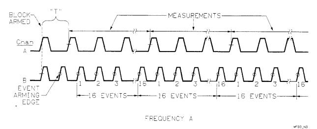
Figure 2-17. Frequency | Edge/Cycle
