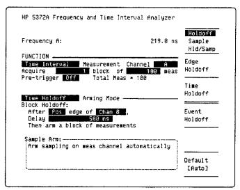
The term, "Block Holdoff," implies that there is some condition which must be satisfied before the Analyzer can begin to collect measurement samples. This is continuous arming.
