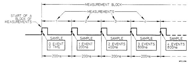
Figure 2-1. Measurements are Made from Samples
