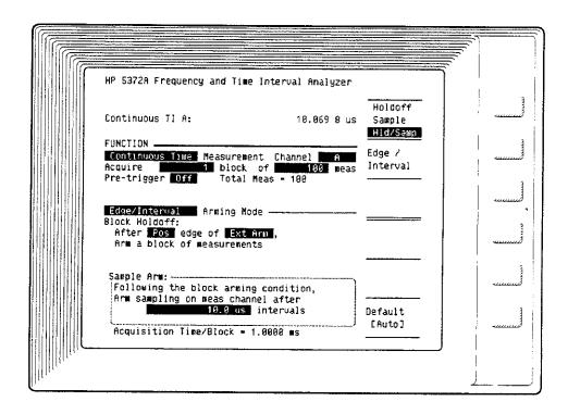
MEASUREMENTS: Time Interval, Continuous Time Interval, ± Time Interval, Frequency, Period, Totalize, Phase, Phase Deviation, and Time Deviation
