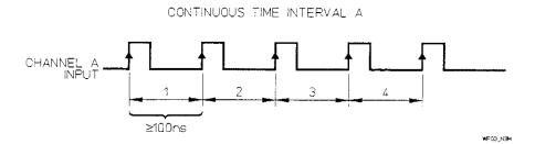
Continuous Time Interval is similar to a Period measurement, but CTI never provides the average time interval when a measurement occurs over more than one period of the signal. A CTI result is the time over which the measurement was made. A Period result is the average of the signal periods that occur during the time of the measurement. *Figure 1-5* compares CTI and Period measurements.
