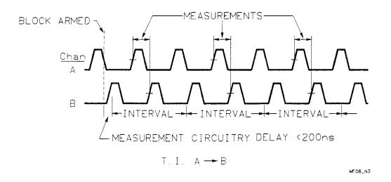
Figure 1-21. Time Interval | Interval Sampling
