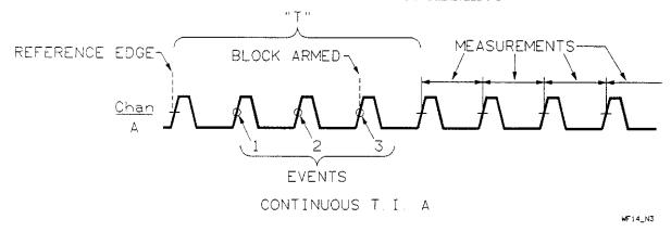
Figure 1-29. Continuous Time Interval | Event Holdoff
