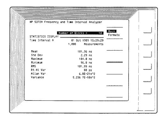
The Statistics Display shows eight statistical results. Statistics are enabled on the Math menu. The values are computed for each block of measurements. When the number of blocks is set greater than one, the statistics include the total number of measurements.
