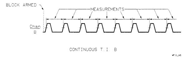
Figure 1-26. Continuous Time Interval | Automatic
