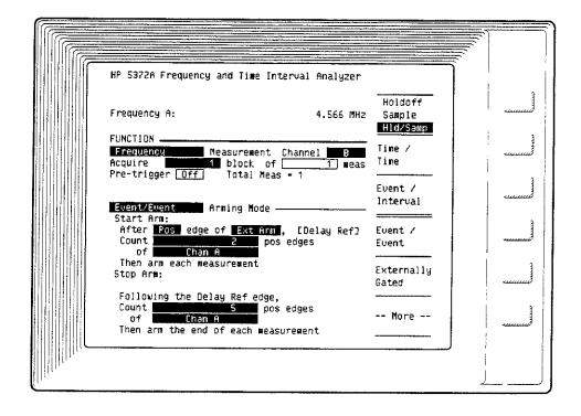
MEASUREMENTS: ± Time Interval, Frequency, and Period
