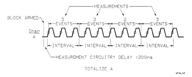
Figure 3-1. Totalize | Interval Sampling
