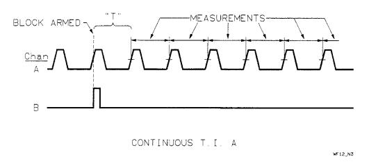
Figure 1-27. Continuous Time Interval | Edge Holdoff
