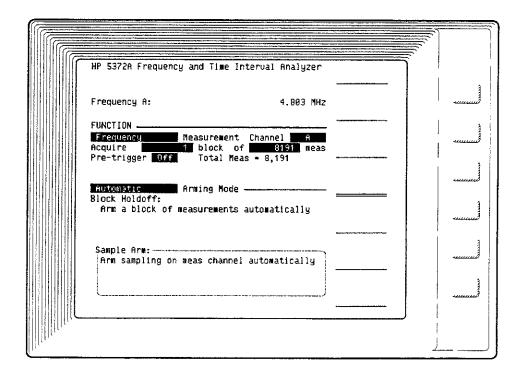
When the number of blocks is set to one, every measurement result will be stored in measurement memory and available for review. For the menu shown in *Figure 7-2*, the following results features are available:
