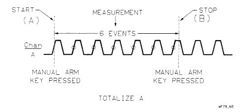
Figure 5-58. MANUAL Timing Diagram
