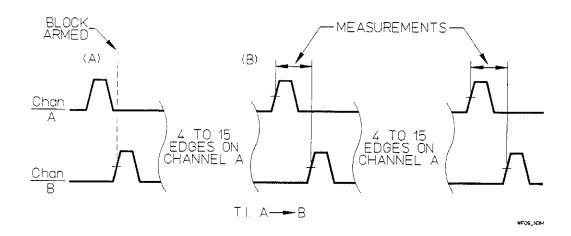
Figure 5-46. EDGE/RANDOM Timing Diagram
