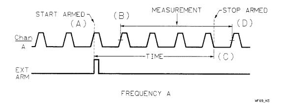
Figure 5-36. EDGE/TIME Timing Diagram
