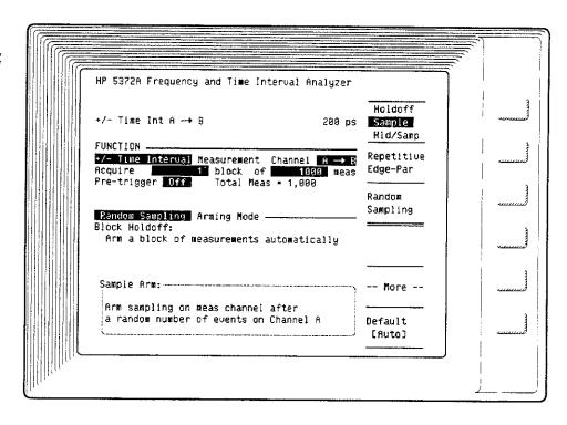
MEASUREMENTS: Time Interval, ± Time Interval
