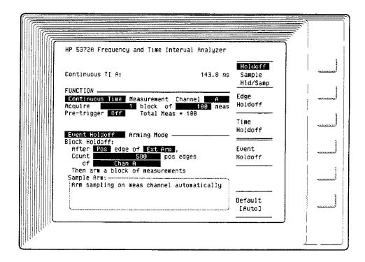
As described on the menu, after a positive event on External Arm, 500 events will be counted on Channel A before the first measurement sequence begins.
