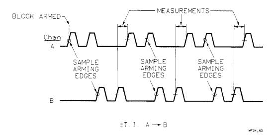
Figure 1-42. ± Time Interval | Edge/Parity
