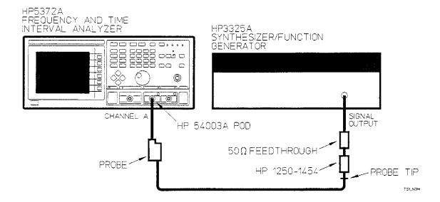
Figure D-1. HP 10017A 10:1 Probe Calibration Setup
