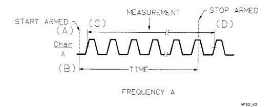
Figure 5-20. TIME SAMPLING Timing Diagram
