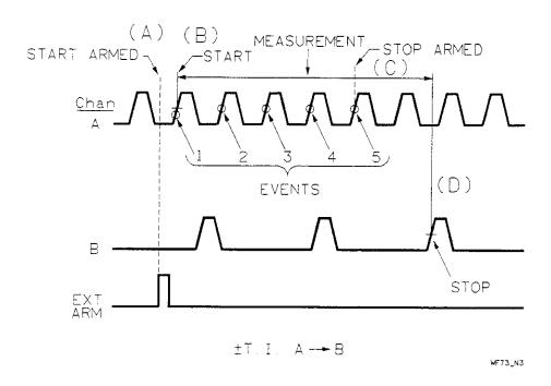
Figure 5-42. EDGE/EVENT Timing Diagram
