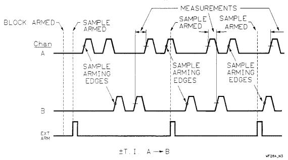
Figure 1-38. ± Time Interval | Repetitive Edge-Parity
