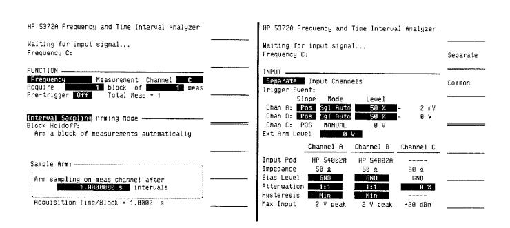
Figure 17-17. Channel C Configuration
