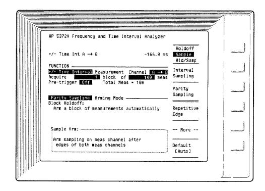
MEASUREMENT: ± Time Interval (two-channel)
