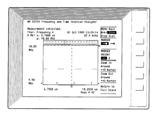
Figure 10-8. Time Interval Measurement With Inhibit
