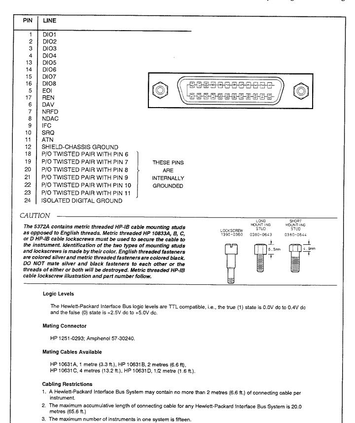
Figure B-2. Hewlett-Packard Interface Bus Connection.
