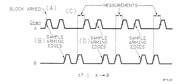
Figure 5-44. EDGE/PARITY Timing Diagram
