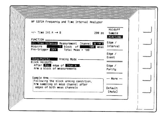
MEASUREMENT: ± Time Interval (two-channel)
