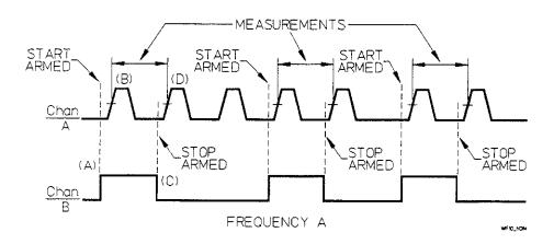
Figure 5-56. EXTERNALLY GATED Timing Diagram
