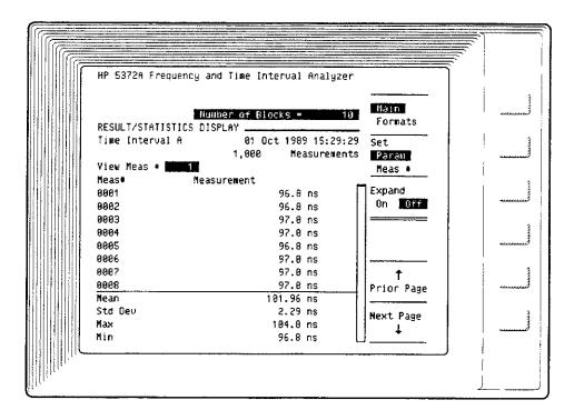
This screen is a combination of the previous two displays. Fewer measurements and statistics values are listed here. The softkey options are the same as for the Result Display.
