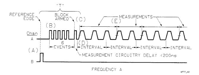
Figure 5-52. EVENT/INTERVAL Timing Diagram
