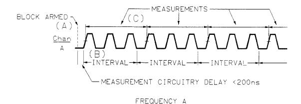
Figure 5-18. INTERVAL SAMPLING Timing Diagram
