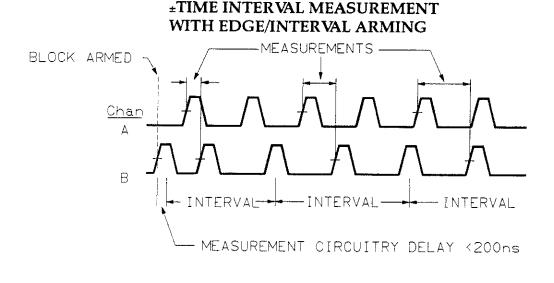
Figure 1-40. ±Time Interval | Edge/Interval
