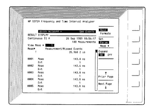
The Numeric screen shows that one event was missed for each measurement. For CTI measurements, this means that one event was not timed during each measurement, but was included in the measurement. Notice the time listed before the first measurement. It is preceded by a "T". This is the time from the occurrence of the event on External Arm to when the first measurement sample is acquired. For this example, "T" is the time for 500 events.
