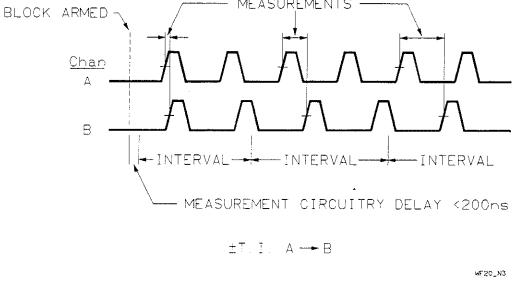
Figure 1-35. ± Time Interval | Interval Sampling
