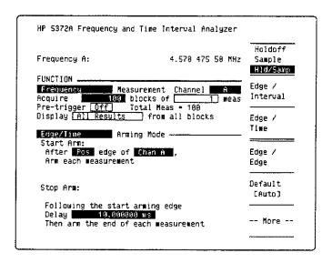
Measurements will be collected one at a time. For example, 100 blocks of 1 measurement. Each measurement will have a discrete start and stop. This is an example of a non-continuous arming process.
