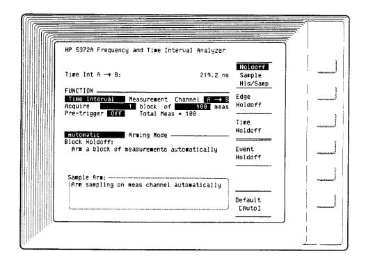
MEASUREMENTS: Time Interval, Continuous Time Interval, ± Time Interval, Frequency, Period, Phase, Phase Deviation, and Time Deviation
