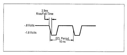
Measurement uncertainty example using Time Interval to measure from falling edge to falling edge of an ECL signal.
