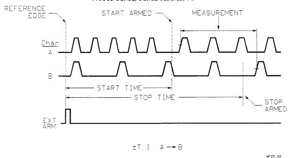
Figure 1-43. ±Time Interval | Time/Time
