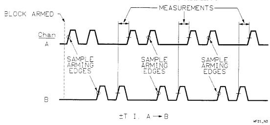
Figure 1-36. ±Time Interval | Parity Sampling
