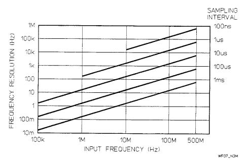
For example, taking samples at 100  $\mu$ s intervals on a 10 MHz input signal will yield a result resolved to 10 Hz (10. 000 00 MHz).
