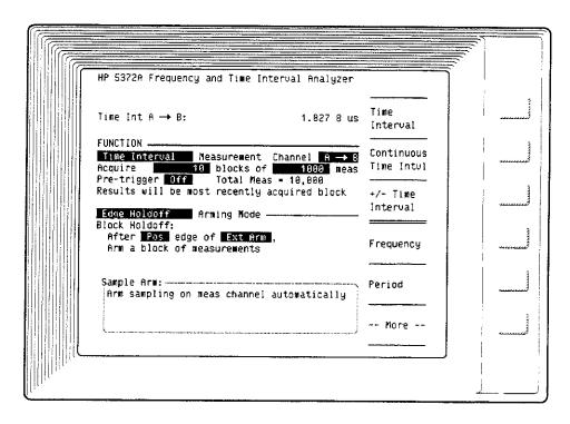
■ UPDATE While — the Histogram is updated after each block to reflect the cumulative data. This mode is sometimes referred to as a "growing histogram." It is useful for observing trends after only a few blocks to help determine if the measurement is appropriate.
