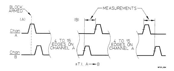
Figure 5-32. RANDOM SAMPLING Timing Diagram
