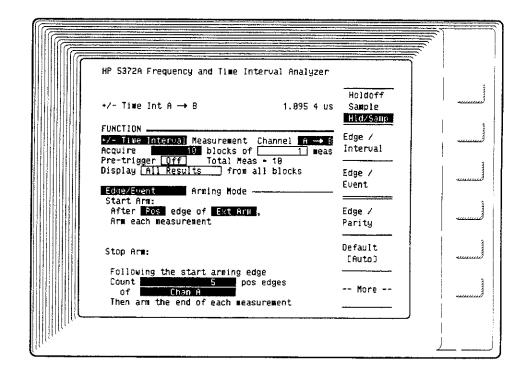
MEASUREMENTS: ±Time Interval, Frequency, and Period
