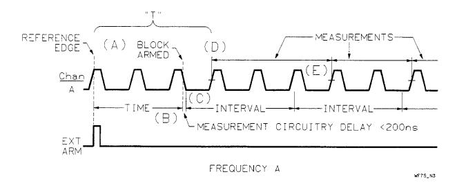
Figure 5-48. TIME/INTERVAL Timing Diagram
