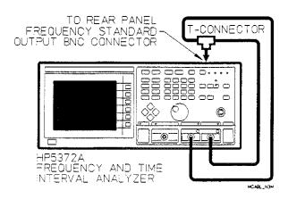
Figure 17-1. HP 5372A Operation Verification Setup
