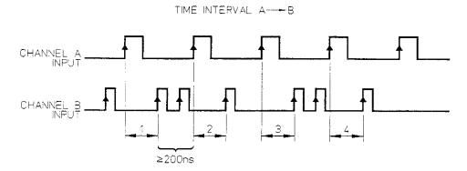
NCTE THAT MEASUREMENTS ALWAYS START ON THE CHANNEL A SIGNAL
