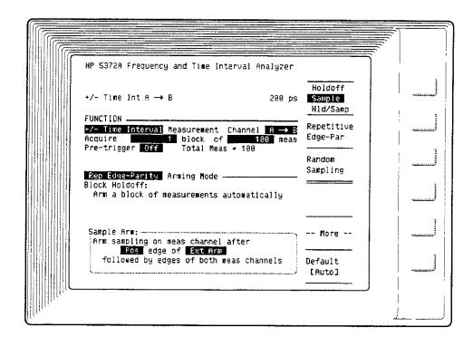
MEASUREMENTS: ± Time Interval (two-channel)
