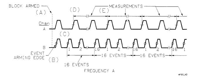
Figure 5-22. CYCLE SAMPLING Timing Diagram
