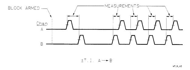
Figure 1-33. ± Time Interval | Automatic
