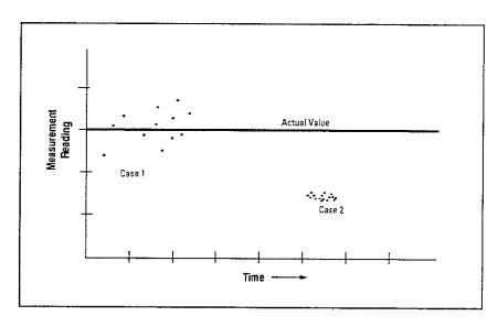
Case 1 shows the results of random uncertainties (resolution) limiting measurement precision. Case 2 shows the results of systematic uncertainty limiting measurement precision. Accuracy specifications must include both systematic and random effects.
