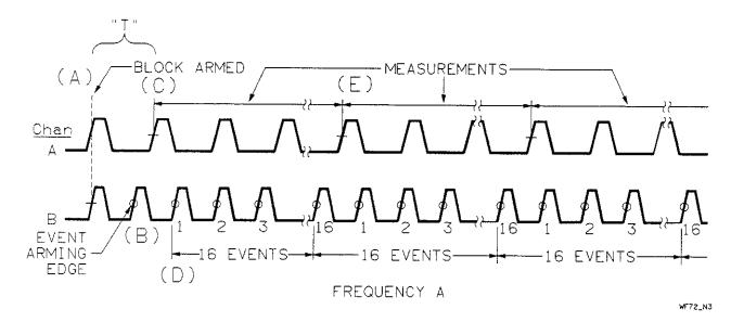
Figure 5-40. EDGE/CYCLE Timing Diagram
