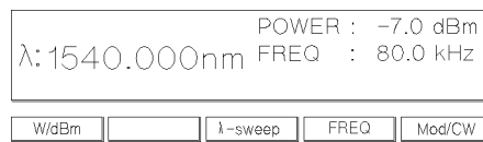
Figure 2-9. Setting the Output Power of an Internally Modulated Signal
