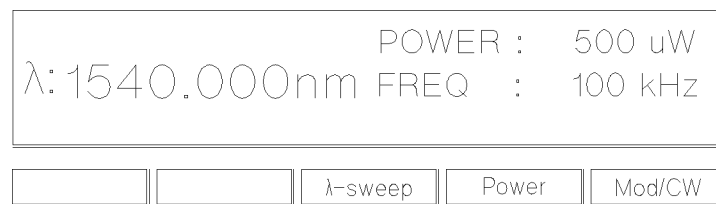
Figure 1-8. Tunable Laser Source Display after Setting Up Wavelength and Power
