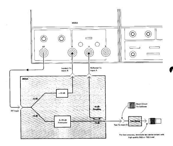
Connections to the test set and test device are made using the cables supplied in the 11851A Cable Kit. The test device input port is connected to the 8502 front panel TEST connector. For reflection calibration, connect the short circuit at the same point to which the test device will be connected. Whatever configuration is used, all cables, adapters, and fixtures required for the measurement should also be used during calibration.
