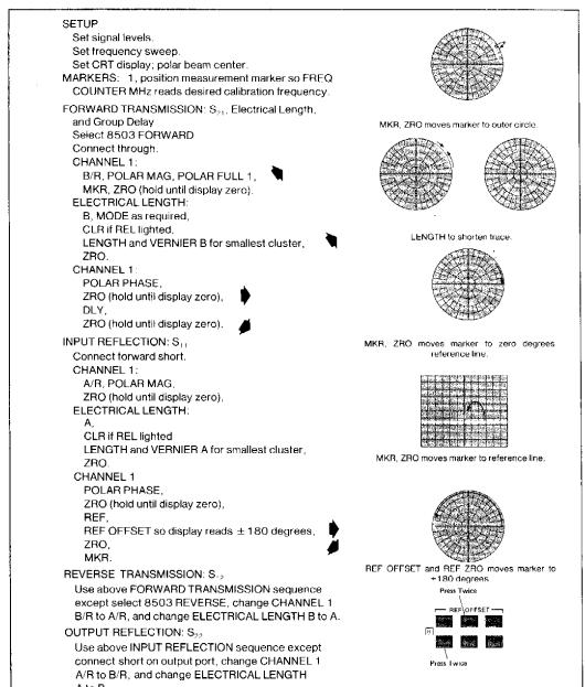
The measured value for any of the S-Parameters can be read directly from the polar display graticule. The magnitude ratio,  $\tau$  for transmission or  $\rho$  for reflection, is read from the concentric circles and the angle.  $\phi$ , read from the radial lines. [Also see page 11].
