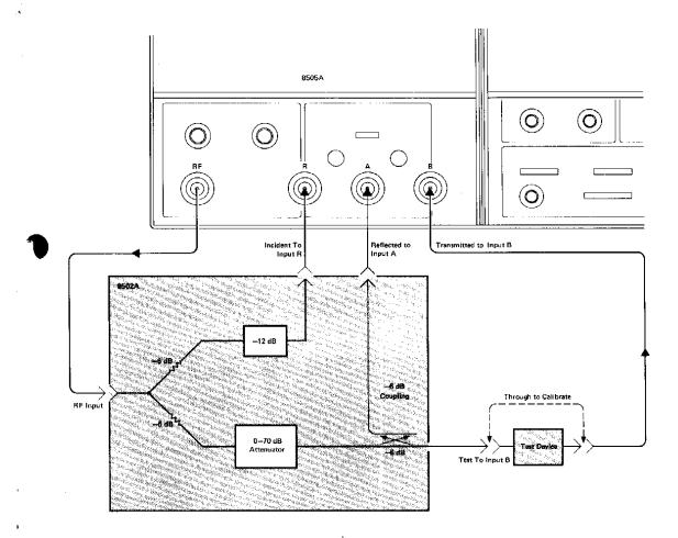
Connections to the test set and test device are made using the cables supplied in the 11851A Cable Kit. The test device input port is connected to the 8502 front panel TEST connector. For transmission calibration, the cable which connects to the device output is connected to the 8502 TEST output. Whatever configuration is used, all cables, adapters, and fixtures required for the measurement should also be used for calibration.
