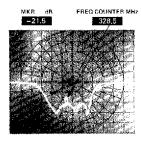
Standing wave ratio, SWR, can be calculated from the return loss measured value using the HP Reflectometer Calculator or these equations:
