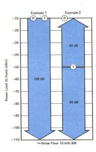
At low signal levels measurement uncertainty is seen as noise on the CRT trace. Select the 1 kHz IF bandwidth (the 1 kHz button to the right of the CRT) to reduce the pre-detection bandwidth and improve the signal-to-noise ratio into the detectors. Select the VIDEO FILTER to reduce the post-detection bandwidth and thus reduce the residual uncertainty caused by detector noise. Slower scan time may be required.
