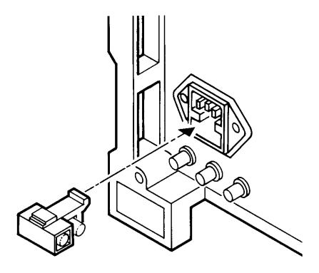
Figure 2-3. Checking the Line Fuse
