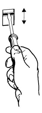
Figure 2-2. Setting the Voltage Selector Switch
