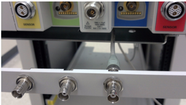
Figure 1-27 Connect the BNC connector to the bottom trim plate
