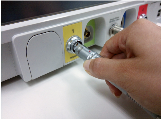
Figure 1-11 Connecting the sensor cable to the 8990B
