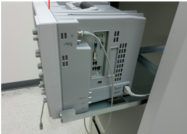
Figure 1-28 Notch at the 8990B to fit the top trim plate
