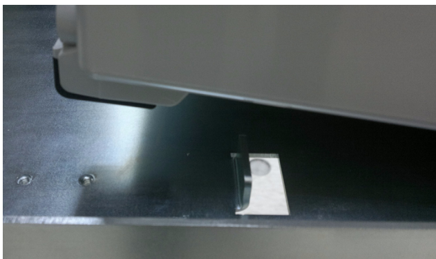
Figure 1-21 Raised tabs in the support tray
