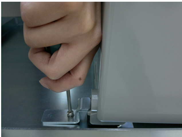
Figure 1-25 T-20 TORX screws
