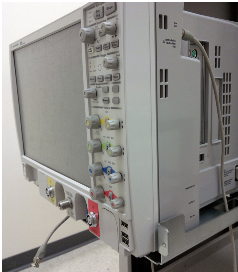
Figure 1-23 BNC connectors to the of the 8990B
