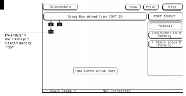
Driving the Port Out BNC in an Intermodule Measurement
