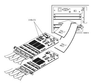
Cable Connections for Two-Card HP 16550A Installations
