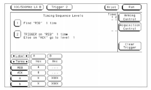
• TRIGGER on "REQ" 1 time Else on "ACK" go to level 1
