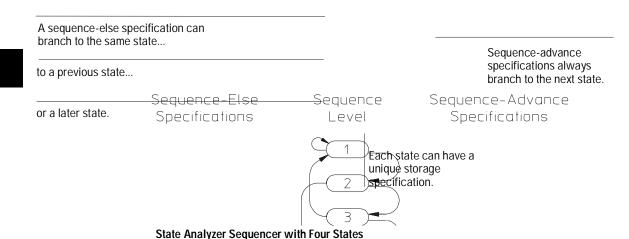
Each state, except for the last, has two branch conditions. These are the sequence-advance and sequence-else specification. (The triggeron specification is a special sequence-advance specification that is described in the section "TRIGGER On Specification.")
