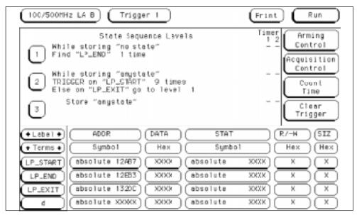
Trigger Setup for Triggering on the 10th Iteration of a Loop
