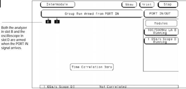
State Analyzer and Oscilloscope armed from PORT IN
