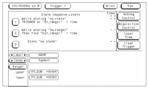
Trigger Setup for Storing Execution of a Subroutine
