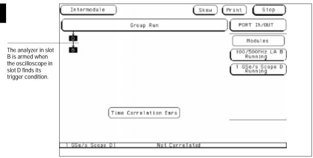
Oscilloscope Arms State Analyzer in Group Run
