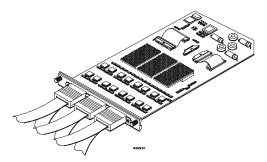
Cable Connections for One-Card HP 16550A Installations
