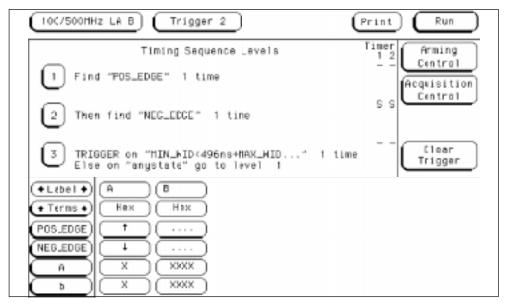
Triggering when a Pulse Exceeds Minimum or Maximum Limits
