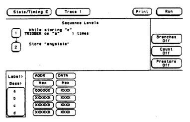
Figure 8-18. State Trace Specification
