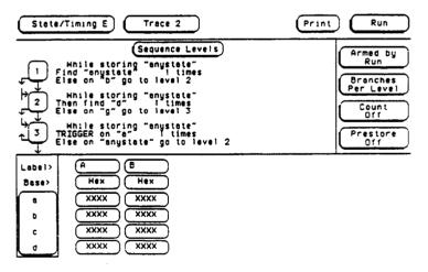
Figure 5-70. Multiple Branching Between Levels
