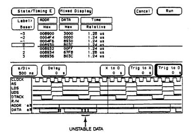
Figure 9-20. Mixed Mode Display with Unstable Data
