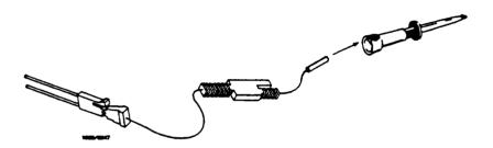
Figure 2-9. Connecting Grabbers to Probes
