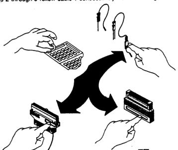
Figure 2-11. Labeling Pods, Probes, and Cables
