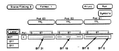
Figure 5-10. Numbering of Assigned Bits
