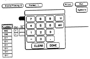
Figure 3-4. Numeric Entry Keypad
