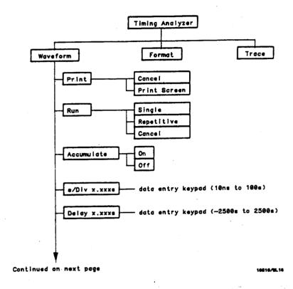
Figure 4-4a. P/O Timing Waveform Menu Map
