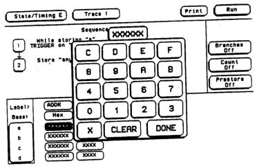
Figure 8-16. Address Pattern Selection Keypad
