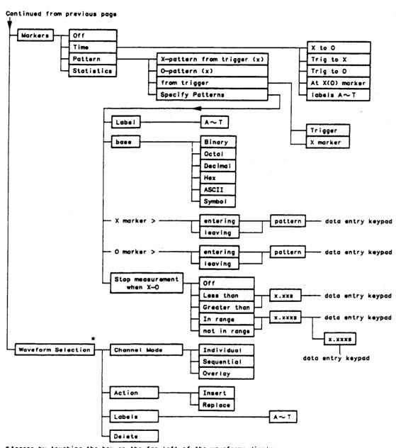
\*Access by touching the box on the far left of the waveforms display where the labels are displayed
