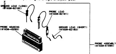
Figure 2-3. Probe Assembly 1850/EX44
