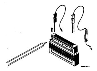
Figure 2-8. Disconnecting Probes from Pods
