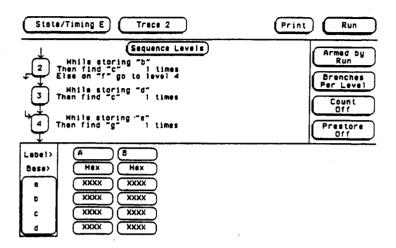
Figure 5-69. Branching Between Sequence Levels
