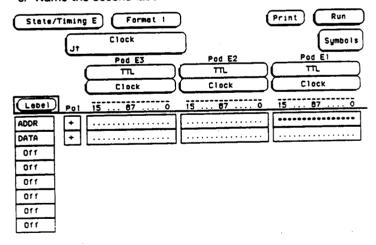
Figure 8-5. State Format Specification with Labels Assigned
