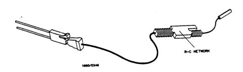
Figure 2-4. Probe Cable
