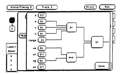
Figure 5-51. Patterns Assigned for Logical Combinations
