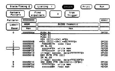
Figure 11-2. Inverse Assemble Field
