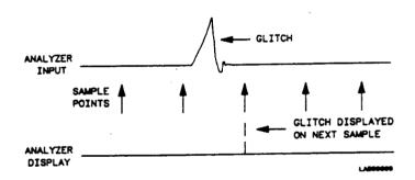
Figure 5-34. Glitch in Timing Waveform
