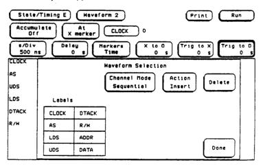
Figure 9-11. Waveform Selection Menu Labels
