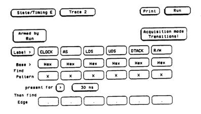
Figure 9-7. Timing Trace Specification Menu
