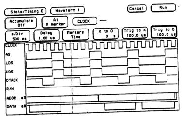
Figure 6-9. Trigger and Trace Points
