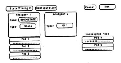
Figure 9-1. State/Timing E Configuration Menu
