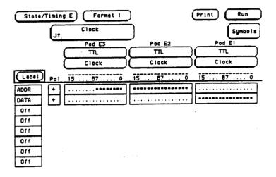
Figure 8-8. State Format Specification Menu with Bits Assigned
