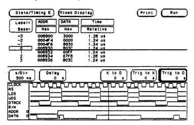
Figure 6-15. Timing/State Mixed Mode Display
