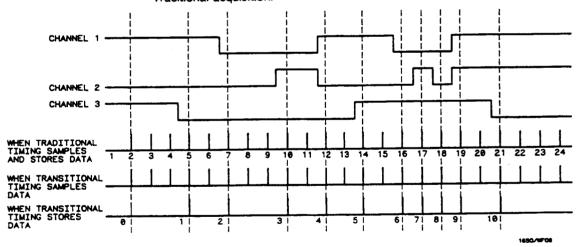
Figure 5-32. Transitional Timing vs. Traditional Timing
