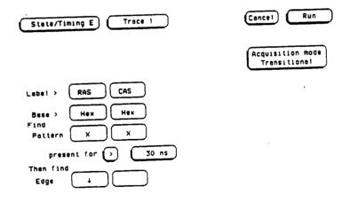
Figure 7-5. Timing Trace Specification Menu
