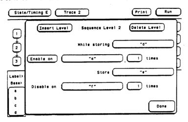
Figure 5-60. Storage Macro Sequence Level Example
