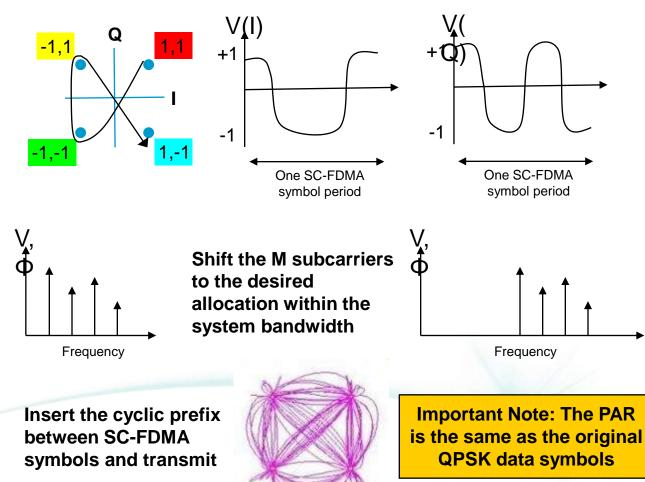
Perform a DFT of length M and sample rate M/(symbol period) to create M FFT bins spaced by 15 kHz
