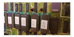
Very carefully I started removing the adapters. Even though HP made quite sturdy PCBs, I didn't want to risk any more damage, so I snipped the pins of the adapters and removed them one by one. I also removed the two 74Is373, they are the ones with the two jumpers next to them. You can see the solder blobs at their ends near to the EPROMs. That is where their pins were snipped and soldered from above, presumably to fit after the adapter boards were already put in.
