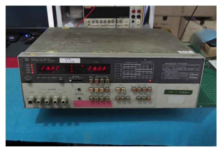
Initial checks quickly revealed absence of negative -12V supply. And because of that there are no negative bias voltage available to processor, which prevents digital controller to work. Usual approach to diagnose and repair power supply issues first pays off once again. It's very good rule to start with visual inspection and DMM checks on unknown condition instrument, starting with power supply circuits.
