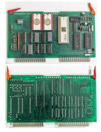
This instrument is using unique **Nanoprocessor** designed by HP Loveland Instrument Division using NMOS process. It's an 8-bit processor optimized for instrument control. It has an 11 bit program counter, one 8 bit accumulator and 16 8-bit storage registers with a grand total of 42 instructions. This processor used in a number of instruments and GPIB controllers by HP.
