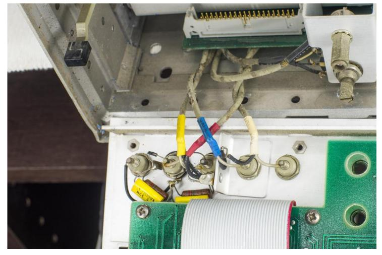
Front panel fully disassembled and washed intensively in hot soapy water with considerable amount of brushing:
