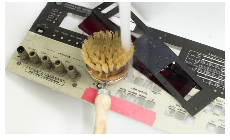
One of binding posts terminals have damaged housing and unable to fix securely on front panel frame. So it was decided to replace custom HP-specific binding post terminal and other three of them to new isolated BNC connectors. Most of modern LCR meters and fixtures are designed to use BNC-style connection, so with few limitations this will allow easier use of 4262A with other fixtures and test probes.
