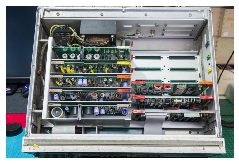
Some of the power supply components are mounted on inner chassis frame, such as transistors Q2 and Q3 in large TO-3 package, and rectifier diodes after primary transformer.
