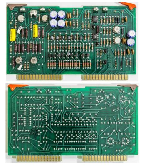
A14 Phase Detector and Integrator PCBA
