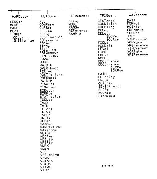
The common commands are commands which are independent of the tree and do not affect the position of the parser within the tree. Root level commands are commands that reside at the root of the command tree. They are prefaced by a colon that puts the parser at the root level. Finally, the subsystem commands are commands that are grouped together under a common node of the tree, such as the TIMEBASE commands.
