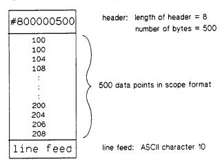
The waveform data inside the oscilloscope can be transferred out in a variety of formats. The data is in a defined block format with a header specifying the length of the block. The block is terminated with a line feed character (ASCII character 10).
