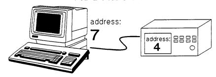
DEVICE ADDRESS = (Interface \* 100) + Instrument
