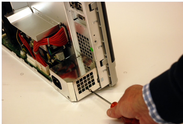
Figure 26 Removing the AC input shield
