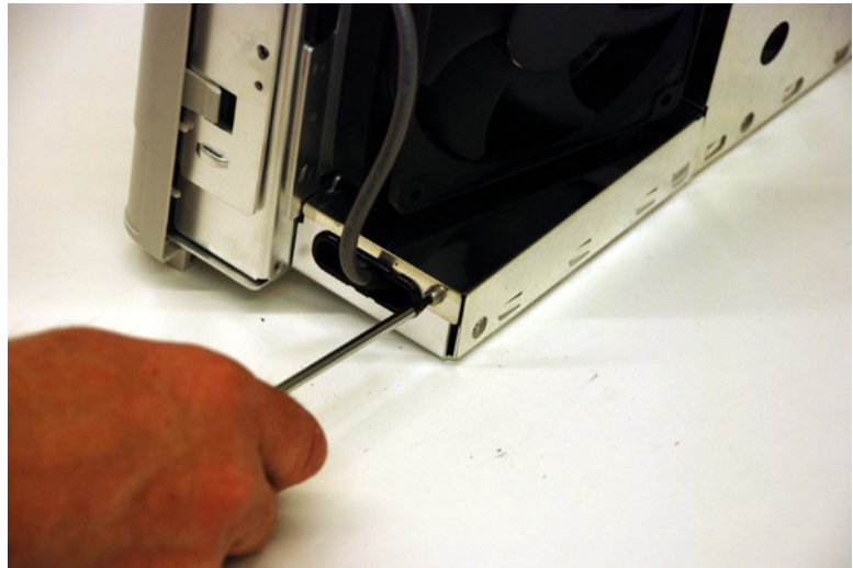
Figure 25 Removing the probe power shield
