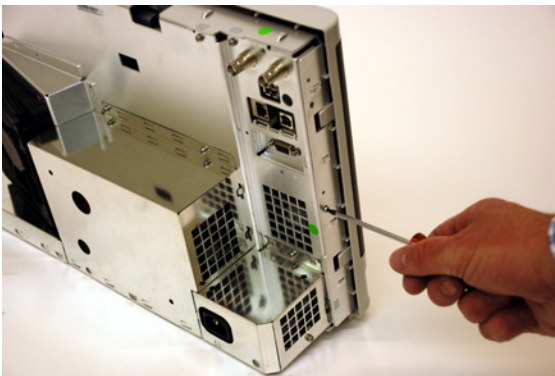
Figure 20 Removing perimeter screws securing rear deck
