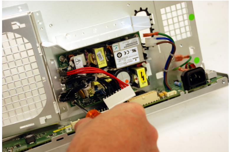
Figure 46 Removing the power supply
