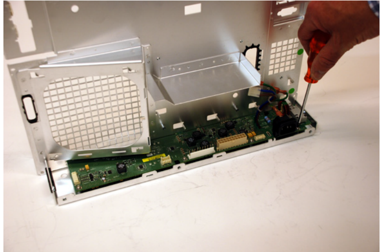
Figure 48 Removing the power board
