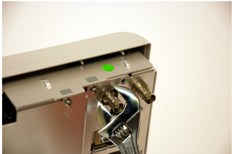
Figure 19 Removing the BNC securing nuts and washers
