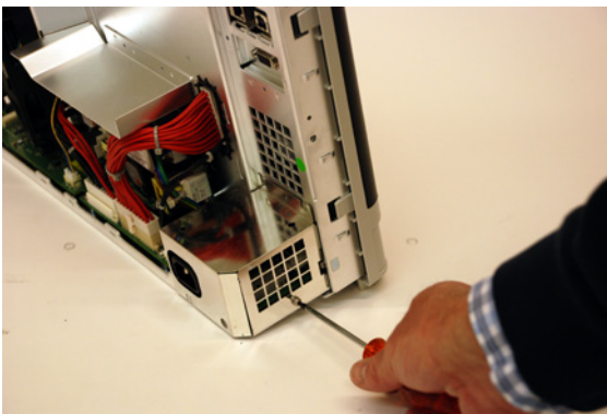
Figure 21 Removing rear-facing screws securing rear deck
