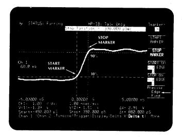
This alternative is considered to be more accurate than the previous two. When we make a pulsewidth measurement in the following experiment, you will see why. Now, return both the delta t and the delta V markers to center screen.
