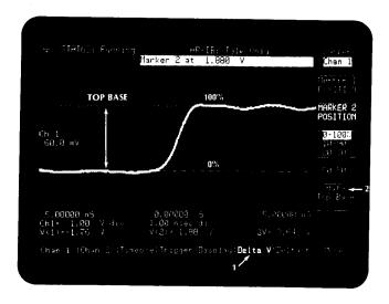
The AUTO TOP-BASE key automatically locates the top and base of the waveform. With these voltage levels as a reference, the delta V markers can now be positioned at the 0-100%, 10-90%, or 20-80% levels by toggling the indicated softkey.
