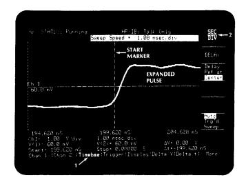
Change the SEC/DIV for several pulses on screen and note that the stop marker comes back on screen at the left.
