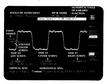
Press TRG'D SWEEP and remove the signal from channel 1. Note that the status is AWAITING TRIGGER, and that the last sweep remains on screen.
