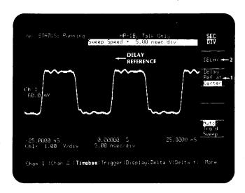
Press the left arrow key repeatedly and note the DELAY= above the graticule. We are moving downstream from the trigger point, just as a conventional scope does when delayed sweep is used.
