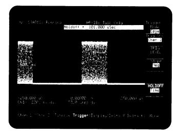
Expand the TIME/DIV to 50 ns/div to see the first few pulses in the burst.
