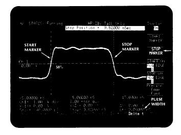
The delta t reading at the bottom of the screen is the pulse width.
