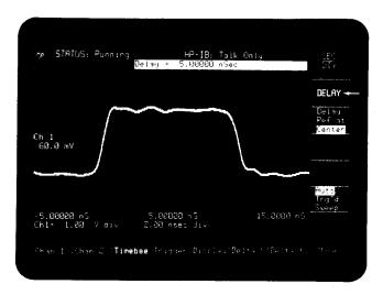
The delta V markers must be positioned at the 50% level as a reference for the delta t markers. Press DELTA V, turn the markers on, and press AUTO TOP-BASE.
