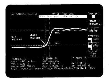
Press STOP MARKER and adjust it to intersect the delta V stop marker (90% point).
