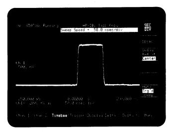
Decrease the **DISPLAY TIME** to 200 ms. Note the very high throughput, resulting in an easy-to-view, dynamic display. Change the pulse height and note the display changes instantly.
