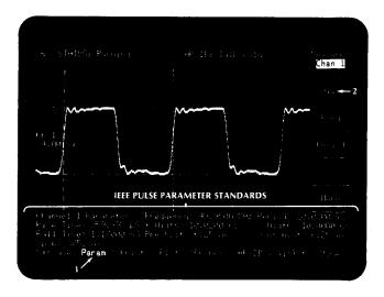
In just a few seconds, you have fully characterized a waveform with nine different parameters—a job that would have required several minutes using a conventional scope. Also, the measurements were made with a high degree of accuracy, totally
