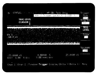
Press the SLOPE POS/SLOPE NEG key and change the edge selected for triggering. Note that the point of reference is center screen. The point of reference can also be to the left or right of the screen. To change the reference, press TIMEBASE and DELAY REF AT CENTER/RIGHT/LEFT. Note the time references changing just below the graticule.
