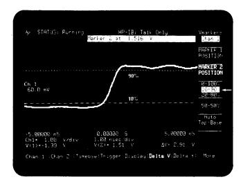
Position the markers on the 10-90% level, press **DELTA** t, and turn the delta t markers on.
