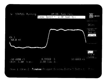
Press DELAY, and adjust it to center the pulse on screen.
