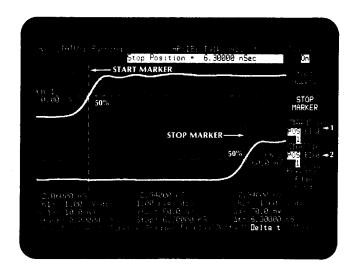
The delta time reading is the extra amount of time required for the signal to travel from channel 1 to channel 2 through the extra length of cable. The time is the electrical length of the second cable.
