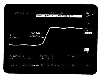
Next, we need to position the delta V markers as a reference for the delta t markers. Press **DELTA V**, turn the markers on, and press **AUTO TOP-BASE**.
