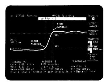
While not as accurate as alternative #3, the operator is not required to find the intersect points as in the previous example. Return both delta t markers to center screen by using the START MARKER, STOP MARKER keys, and the CONTROL KNOB.
