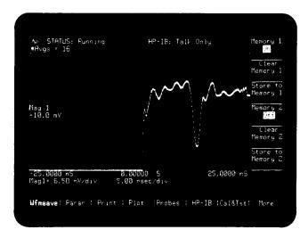
Starting with the probe, remove each of the components up to—but not including—the 50 ohm termination at the end of the cable, restoring the trace after each step. The display should look like the figure. Using the delta V and delta t markers, measure the width and level of the reflection.
