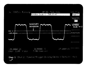
Press POSITION and use the control knob to position the window over the top of the pulses. Turn MAGNIFY ON and observe the display. The steps on the edges are a result of our magnifying the vertical distance between the sample data points, along with the rest of the information inside the magnify WINDOW.
