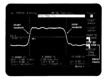
As in the rise-time measurement, the operator is not required to position the markers. Using START MARKER, STOP MARKER, and the control knob, return the two delta t markers to center screen.
