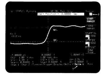
Press START MARKER and adjust the control knob to intersect the delta t start marker with the delta V start marker (10% level).
