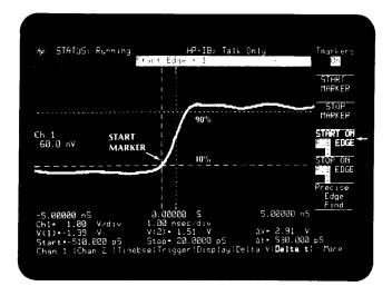
Press STOP ON POS EDGE 1 and note that the delta t stop marker jumps to the 90% point.
