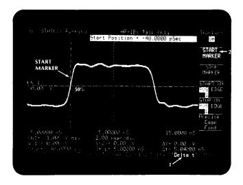
Press STOP MARKER and position it to intersect with the delta V markers at the trailing edge of the pulse.
