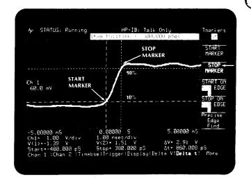
The delta time reading at the bottom of the screen is the rise time between the 10-90% points. Note that the start markers are represented by long dashes, while the stop markers are the shorter dashes. Return both delta t markers to center screen.
