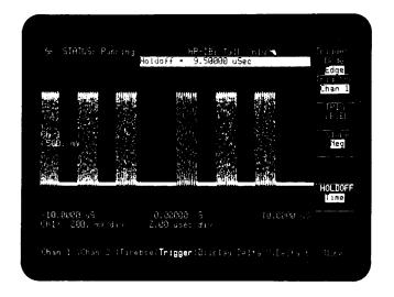
Now we're ready to make a time-interval measurement. First, press DELTA V, then toggle the menu to V MARKERS CHAN 1. Press AUTO TOP-BASE, then 50-50%. This positions both voltage markers at the 50% level of the waveform.
