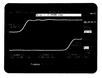
Next, we need to set the delta V markers. We will position them at the 50% points as we did while making the pulse-width measurement. Press DELTA V and toggle the V MARKER key until it reads CH 1 & 2. With the MARKER 1 POSITION turned on, position the marker at the 50% level of the leading edge on channel 1. Press MARKER 2 POSITION and set that marker to the corresponding point of the edge on channel 2.
