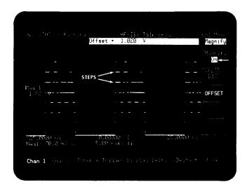
We can eliminate the steps by placing the display in the averaged mode. Press **DISPLAY** and toggle the **DISPLAY MODE** to **AVERAGED**. The number of averages can be varied from 1 to 2048.
