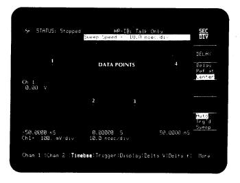
Press DELTA t, and place the markers on two adjacent points. The delta time reading should be approximately 24.6 ns. This is the digitizing sample rate of the HP 54100A/D.
