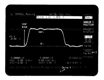
Press the 50-50% key, and note that the markers move to the 50% point of the pulse.
