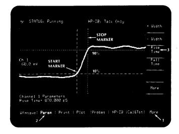
Using this alternative, we are not required to set any of the markers, because all four of them automatically find their respective positions. If the standard 10-90% rise time is the desired measurement, this is the preferred technique.
