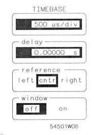
Setting the timebase displays the signal at different time/division settings (Remember the frequency of the HP 54502A is different than the HP 54501A and HP 54503A and will have different values displayed.)
