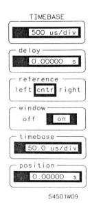
This procedure uses the TIMEBASE WINDOW function to measure the risetime of the signal generator output.
