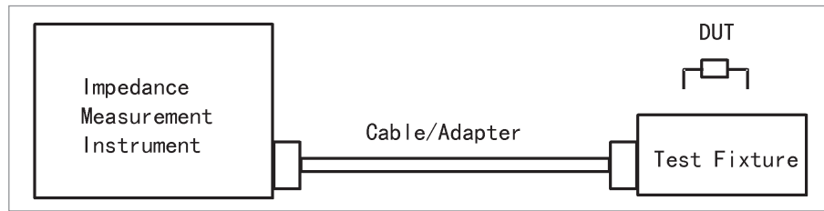
System configuration for impedance measurement
