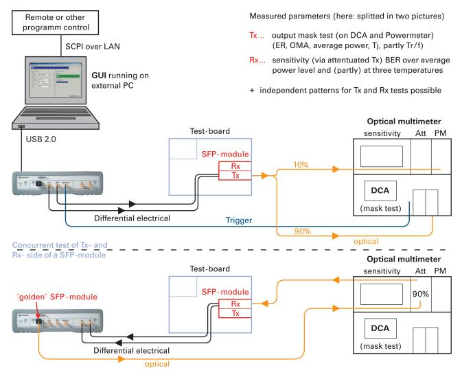
Figure 2: Typical manufacturing tests of SFP-modules
