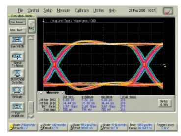
Figure 3: Typical eye diagram at 2.66 Gb/s
