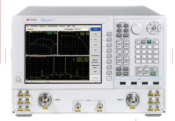
**PNA Network Analyzers:** E8362/3/4B, E8361A 10 MHz to 20, 40, 50, 67, or 110 GHz
