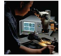
Use TRL calibration for accurate in-fixture, on-wafer, or waveguide measurements.
