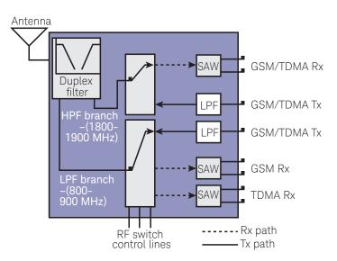
Tri-band antenna switch module with balanced and single-ended ports.
