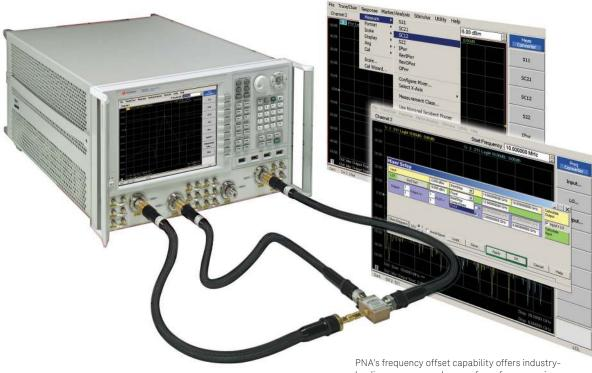
PNA's frequency offset capability offers industryleading accuracy and ease-of-use for measuring mixers and frequency converters.
