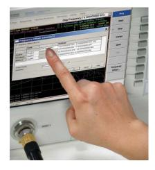
The PNA-X integrates a 10.4 inch high resolution display with a touch screen, which provides a crisp view and easy access to all data and traces. This enhanced user interface allows intuitive operation and helps you set up complex measurements quickly.
