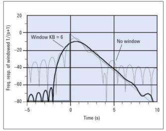
Use time domain to gate out the response of fixtures and cables, and characterize the impedance of transmission lines.
