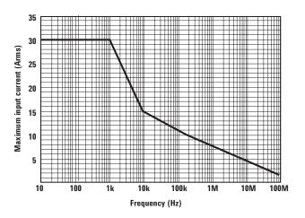
Figure 4. Continuous maximum input rating of N2783B
