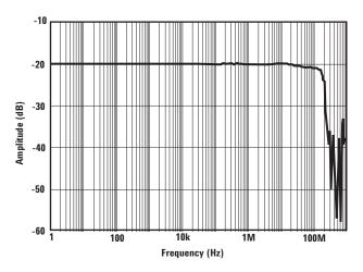
Figure 3. Frequency response of N2783B
