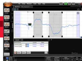
Time domain reflectometer. Measure both impedance and S-parameters, and verify transmission quality on cables, components and channels.
