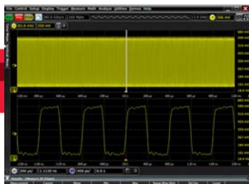
Powerful signal capture. Acquire 25 ms of PCI Express Gen2 data at 40 GSa/s using 1 Gpts of memory to capture your signal of interest.
