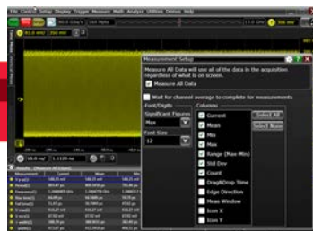
"Measure all edges" mode. Make more than 5 million measurements in less than 1 minute using the "measure all edges" mode and long memory to increase your confidence in the measurement statistics.
