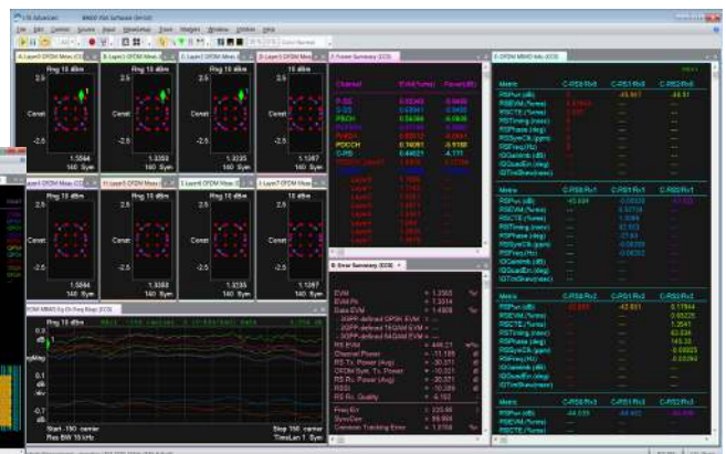
89600 WLA showing LTE-FDD PHY, MAC, RLC and RRC messages with their decoded content.
