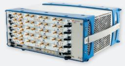
By including five M9703A modules, synchronized using the AXIe bus, this system offers 40 high-speed (1 GS/s) data acquisition channels that look to be one single instrument. Ideal for large scale applied physics experiments such as particle physics, microwave astronomy or hydrodynamics applications.
