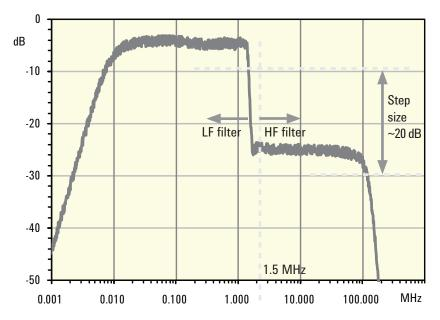
Figure 3. RJ filter noise spectrum for common reference clock architecture with 81150A as noise source
