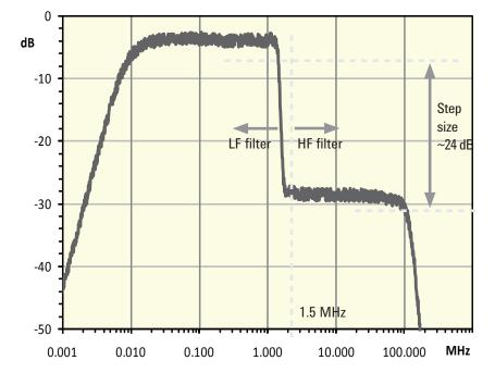
Figure 4. RJ-filter noise spectrum for data clocked architecture with 81150A
