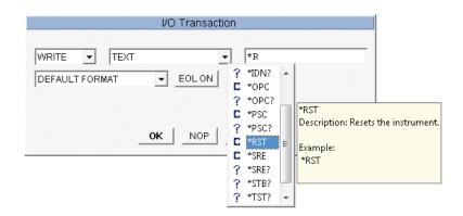
Programming is simplified by capabilities such as auto-completion of SCPI commands, which eliminates the need to memorize command syntax. Simply choose the appropriate SCPI command from the list that appears as you type within the IO Transaction object. A description of the chosen command is also displayed, saving you the trouble of hunting through a manual to check for proper syntax.
