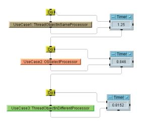
In a multi-core PC, Agilent VEE uses its multi-core programming capability to allocate individual execution threads to different CPU cores, further increasing program performance beyond multithreading alone. The level of improvement varies from application to application.
