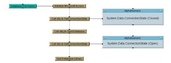
With Agilent VEE, you can easily integrate database operations into your test system. This capability enables connections to databases supported by ADO.NET, including Microsoft Access, SQL Server, Oracle<sup>®</sup> and MySQL. You can store massive amounts of test data in a well-structured format, then retrieve results as needed for additional testing or analysis.
