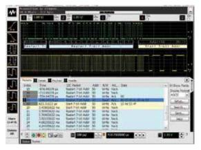
Extend your scope capability with protocol analysis. The tracking marker/bar shows precise time alignment between protocol viewer and analog
