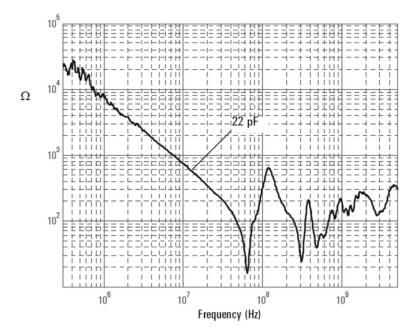
Figure 10. Input impedance vs. frequency of N2791A
