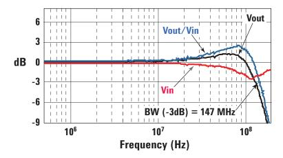
Figure 4. Vout/Vin vs. frequency response of N2790A
