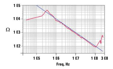
Figure 6. Input impedance vs. frequency of N2790A
