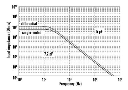
Figure 14. Input impedance vs. Frequency of N2891A
